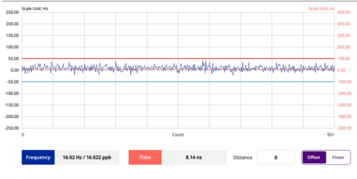
**NOTE:** You can tap the Distance box and input the value that you want to compensate for distance. When distance is entered, the time will show the value with distance correction. Make sure the default value for Distance is 0.
