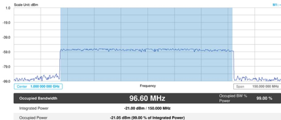
The Occupied Bandwidth measurement shows both of power across the band and power bandwidth in a user specified percentage to determine the amount of spectrum used by a modulated signal. Occupied bandwidth is typically calculated as the bandwidth containing 99% of the transmitted power.
