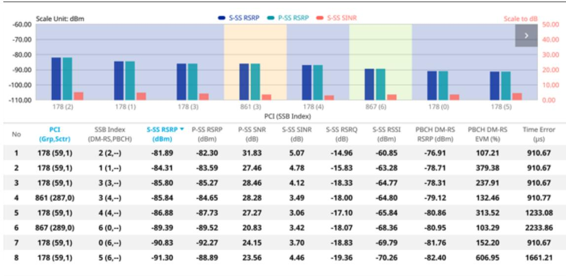
**NOTE:** The undetected values in the Detected ID List table will be indicated as "--". You cannot save the measurement as a Result. Logging as CSV option is added. For more details, see [Managing files](#).
