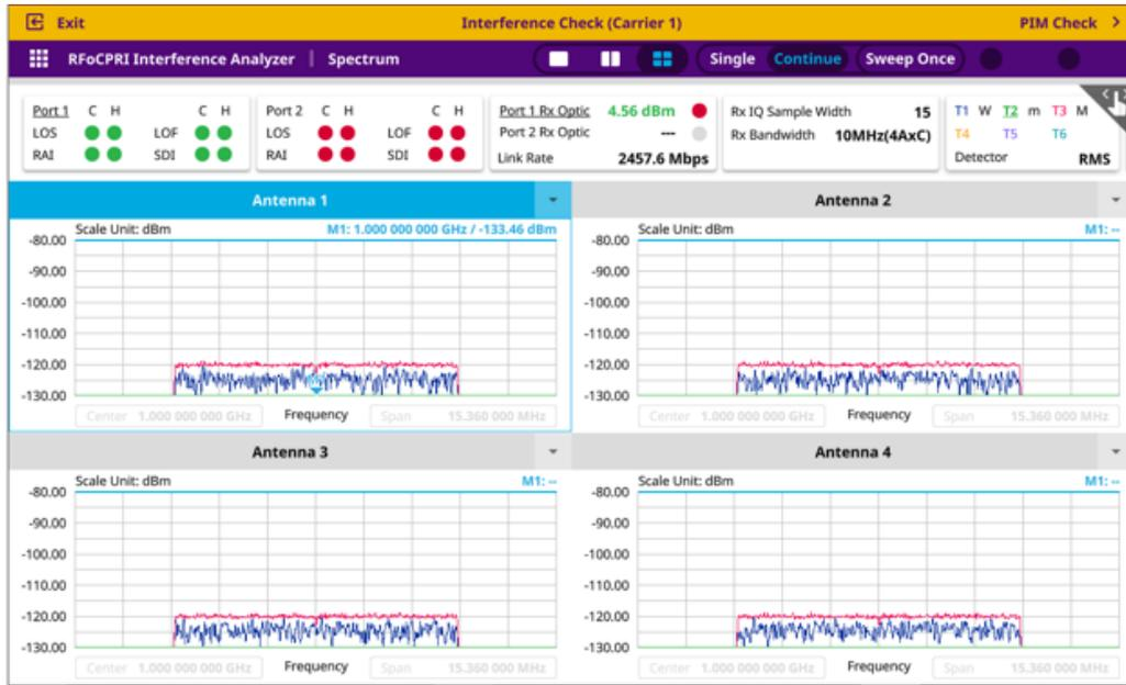
**PIM check chart view with with RFoCPRI Interference Analyzer**
