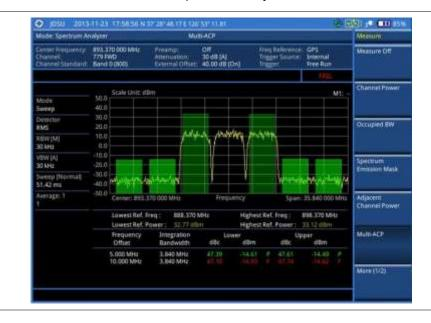
Figure 26 Multi-ACP measurement with spectrum analyzer
