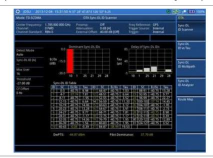
Figure 251 Sync-DL ID scanner measurement with TD-SCDMA OTA signal analyzer
