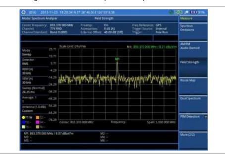
Figure 32 Field strength measurement with spectrum analyzer
