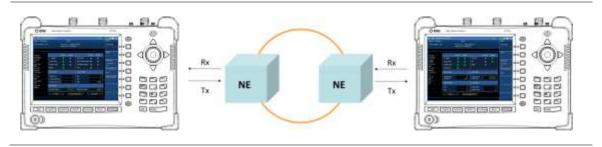
Figure 322 Loop-back connection
