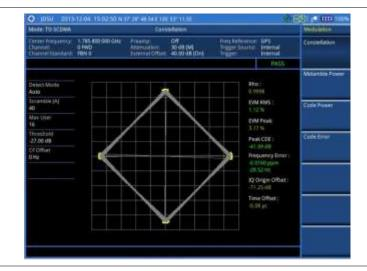
Figure 247 Constellation measurement with TD-SCDMA signal analyzer
