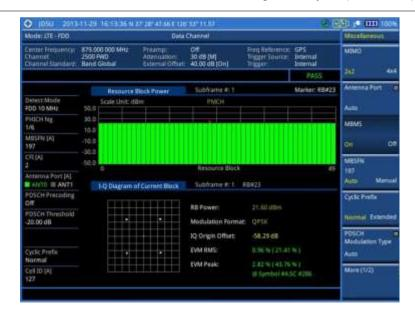
Figure 117 Data channel measurement with LTE - FDD signal analyzer (MBMS On)
