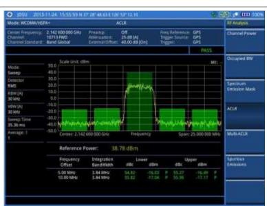
Figure 85 ACLR measurement with WCDMA/HSPA+ signal analyzer
