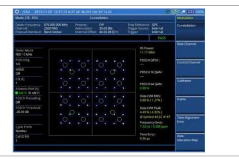
Figure 115 Constellation measurement with LTE - FDD signal analyzer (MBMS On)
