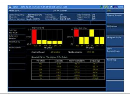
Figure 227 PN scanner measurement with EV-DO OTA signal analyzer
