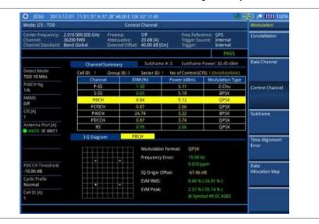
Figure 164 Control channel measurement with LTE - TDD signal analyzer (MBMS On)
