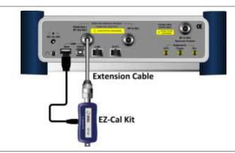
Figure 294 1-port calibration connection with electronic EZ-Cal kit
