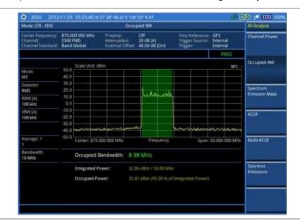
Figure 108 Occupied bandwidth measurement with LTE - FDD signal analyzer
