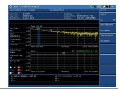
Figure 307 Cable loss (1 port) measurement with the zone enabled
