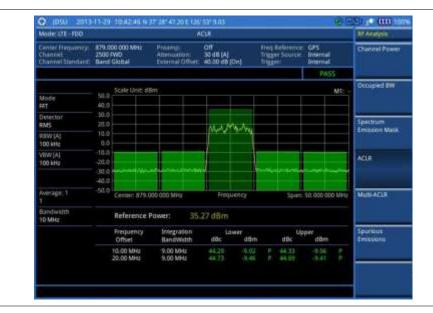
Figure 110 ACLR measurement with LTE - FDD signal analyzer
