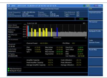
Figure 204 Code domain power measurement with CDMA OTA signal analyzer
