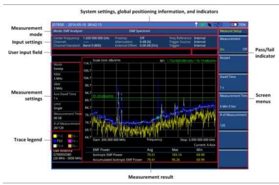
Figure 348 EMF Spectrum measurement screen
