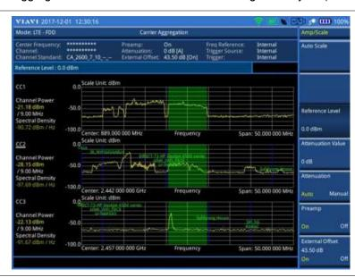
Figure 133 Carrier aggregation measurement with LTE - FDD signal analyzer (SA with Wi-Fi on)
