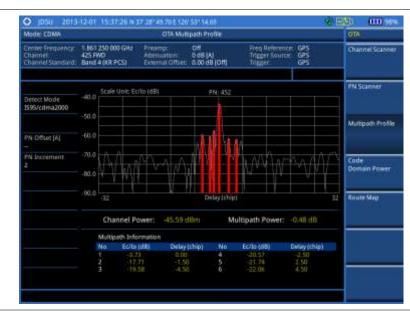
Figure 203 Multipath profile measurement with CDMA OTA signal analyzer
