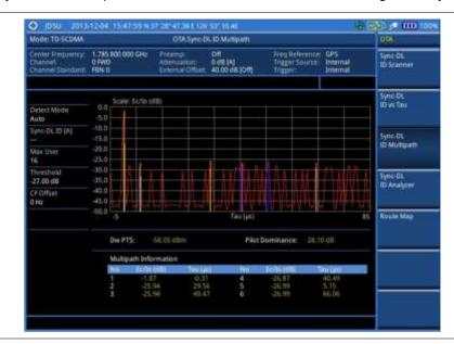
Figure 253 Sync-DL ID multipath measurement with TD-SCDMA OTA signal analyzer
