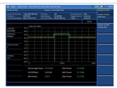
Figure 218 Power vs. time (idle slot) measurement with EV-DO signal analyzer
