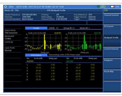
Figure 177 Multipath profile measurement with LTE - TDD OTA signal analyzer
