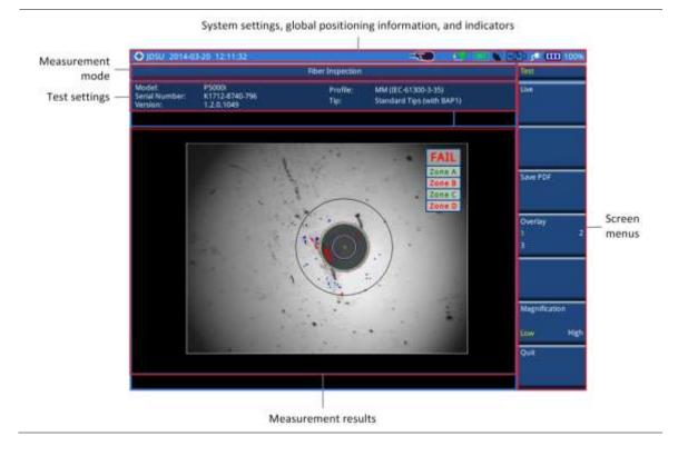
Figure 344 Fiber inspection screen
