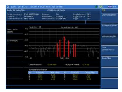
Figure 97 Multipath profile measurement with WCDMA/HSPA+ OTA signal analyzer
