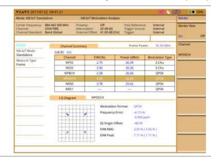
Figure 291 NB-IoT Standalone Modualtion Analysis measurement screen (Subframe 0- NPBCH)
