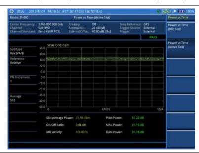
Figure 219 Power vs. time (active slot) measurement with EV-DO signal analyzer
