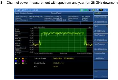
Figure 18 Channel power measurement with spectrum analyzer (on 28 GHz downconverter)
