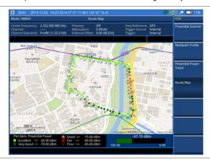
Figure 275 Route map measurement with Mobile WiMAX OTA signal analyzer
