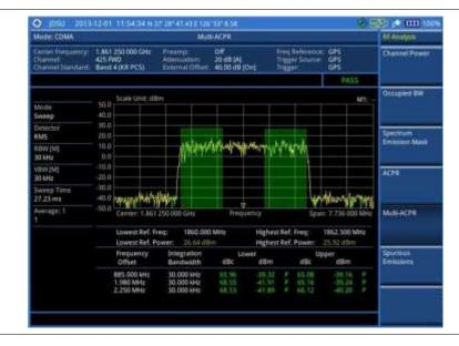
Figure 193 Multi-ACPR measurement with CDMA signal analyzer
