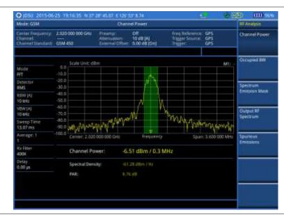
Channel power measurement result shows channel power and spectrum density in a user specified channel bandwidth. The peak to average ratio (PAR) is shown at the bottom of the screen as well. The shaded area on the display indicates the channel bandwidth.
