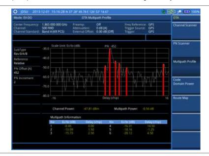
Figure 228 Multipath profile measurement with EV-DO OTA signal analyzer
