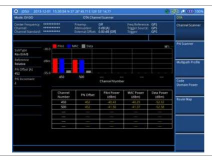
Figure 226 Channel scanner measurement with EV-DO OTA signal analyzer
