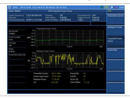
Figure 274 Preamble power trend with Mobile WiMAX OTA signal analyzer
