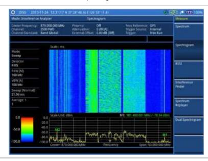
Figure 43 Interference measurement in spectrogram
