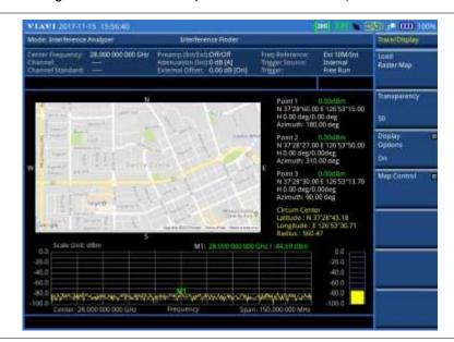
Figure 54 Raster image overlaid on the map in interference finder (on 28 GHz downconverter)
