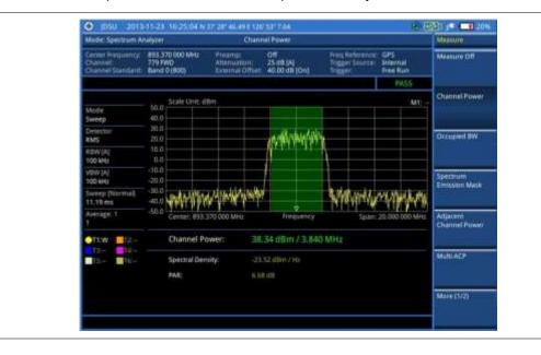
Figure 17 Channel power measurement with spectrum analyzer
