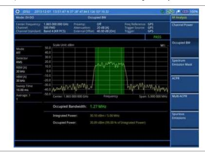
Figure 213 Occupied bandwidth measurement with EV-DO signal analyzer
