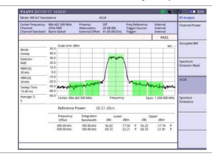
Figure 288 ACLR measurement with NB-IoT Standalond signal analyzer
