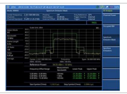
Figure 264 SEM measurement with Mobile WiMAX signal analyzer
