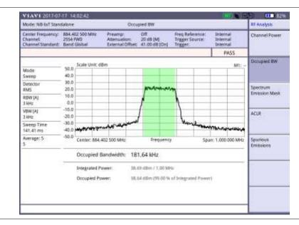
You can use the *LIMIT* hot key to analyze your measurements with the user-definable limit and Pass/Fail indication. See "Setting limit for RF tests" on page 501 for more information.
