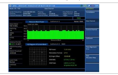
Figure 161 Data channel measurement with LTE - TDD signal analyzer
