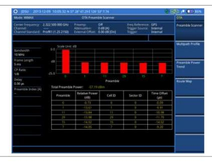
Figure 272 Preamble scanner measurement with Mobile WiMAX OTA signal analyzer
