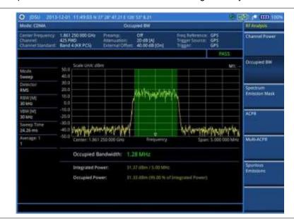
Figure 190 Occupied bandwidth measurement with CDMA signal analyzer
