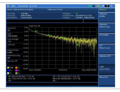
Figure 309 Cable loss (1 port) measurement with zoom
