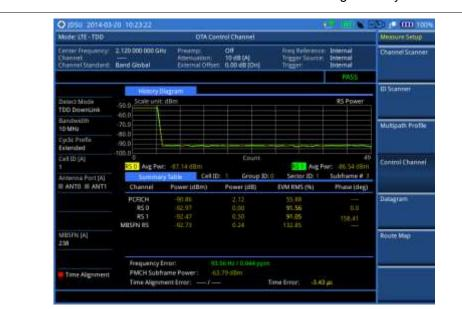
Figure 178 Control channel measurement with LTE - TDD OTA signal analyzer
