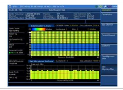
Figure 168 Data allocation map measurement with LTE - TDD signal analyzer
