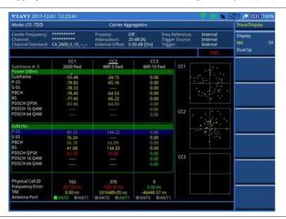
Figure 173 Carrier aggregation measurement with LTE - TDD signal analyzer (SA)
