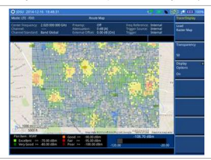
Figure 141 Raster image overlaid on the route map in LTE-FDD OTA signal analyzer
