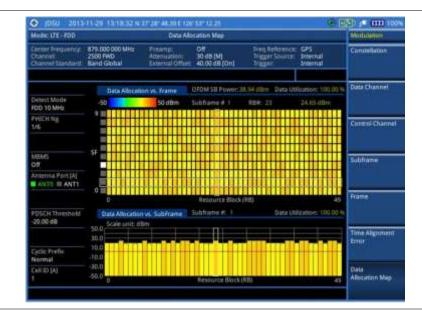
Figure 126 Data allocation map measurement with LTE - FDD signal analyzer
