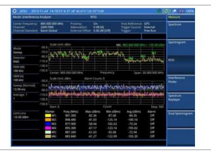
Figure 50 Interference measurement in RSSI (on 28 GHz downconverter)
