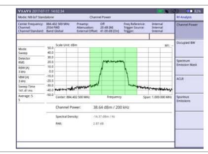
Figure 285 Channel power measurement with NB-IoT Standalone signal analyzer
