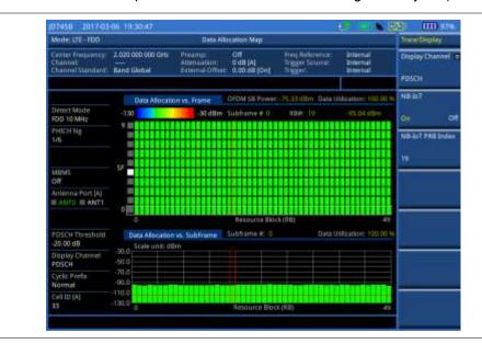
Figure 128 Data allocation map measurement with LTE - FDD signal analyzer (NB-IoT On)
