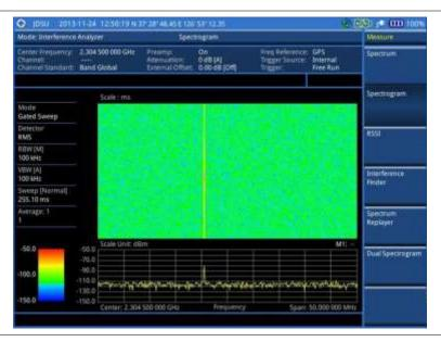
Figure 46 Interference measurement in spectrogram with gated sweep on (on 28 GHz
