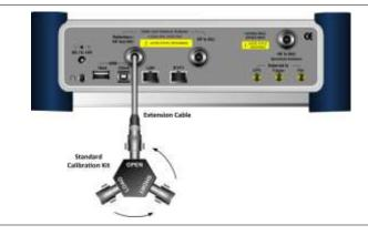
Figure 293 1-port calibration connection with mechanical Y-Cal kit
