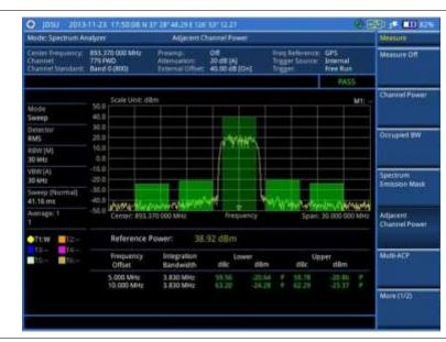
Figure 24 Adjacent channel power measurement with spectrum analyzer
