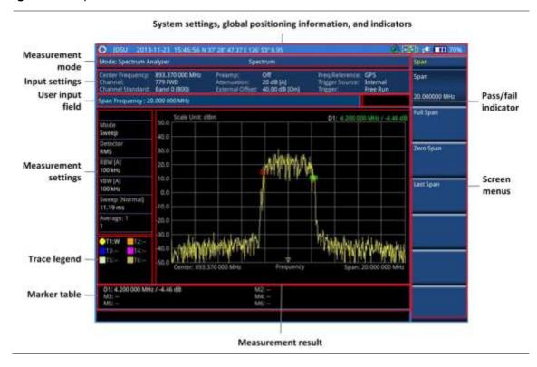
Figure 11 Spectrum measurement screen
