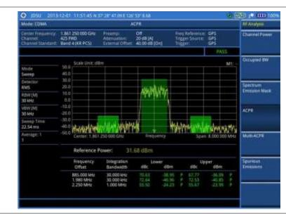
Figure 192 ACPR measurement with CDMA signal analyzer
