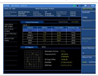
Figure 144 NB-IoT modulation measurement with LTE-FDD signal analyzer (Subframe 2)
