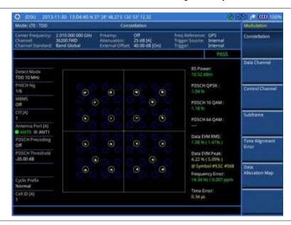
Figure 160 Constellation measurement with LTE - TDD signal analyzer (MBMS On)
