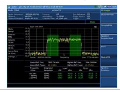
Figure 216 Multi-ACPR measurement with EV-DO signal analyzer
