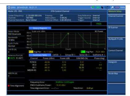
Figure 138 Control channel measurement with LTE - FDD OTA signal analyzer
