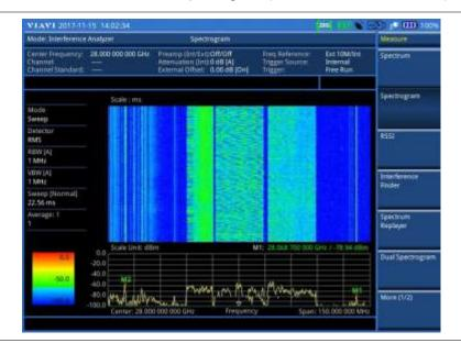
Figure 44 Interference measurement in spectrogram (on 28 GHZ downconverter)
