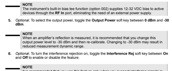
It is recommended that you use this feature only when you suspect interfering signals in the area as turning this on slows down the measurement.
