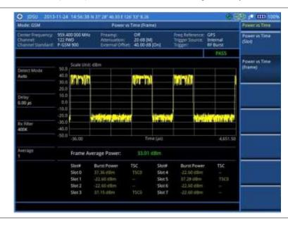
Figure 70 Power vs. time (frame) measurement with GSM signal analyzer
