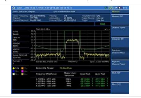
Figure 22 Spectrum emission mask measurement with spectrum analyzer
