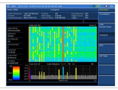
Figure 197 Codogram in full view with CDMA signal analyzer
