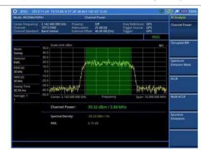
Figure 82 Channel power measurement with WCDMA/HSPA+ signal analyzer
