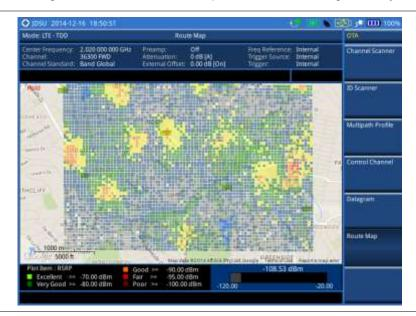
Figure 181 Raster image overlaid on the route map in LTE-TDD OTA signal analyzer
