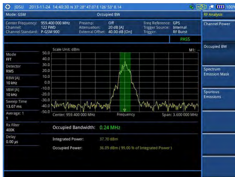
Figure 41 Occupied bandwidth measurement with GSM signal analyzer
