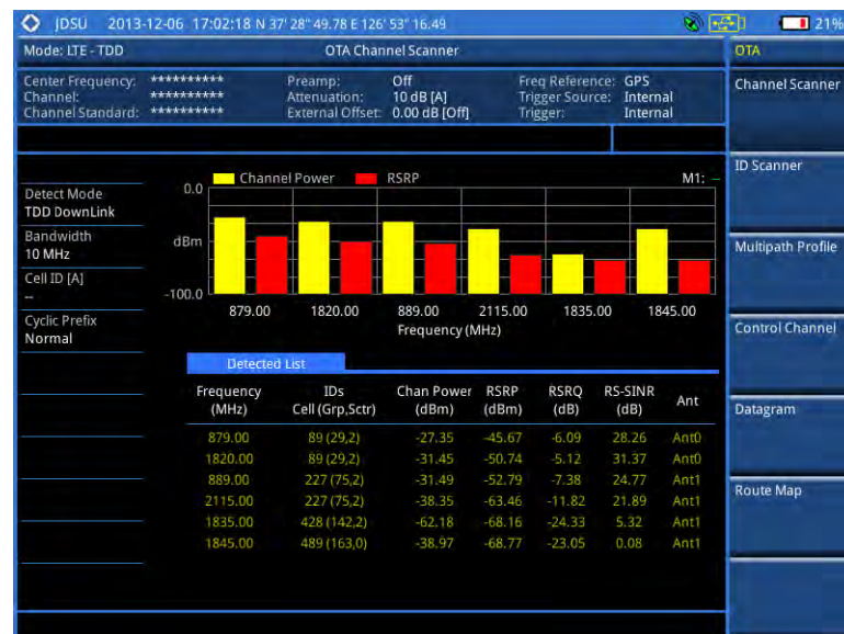
Figure 144 Channel scanner measurement with LTE - TDD OTA signal analyzer
