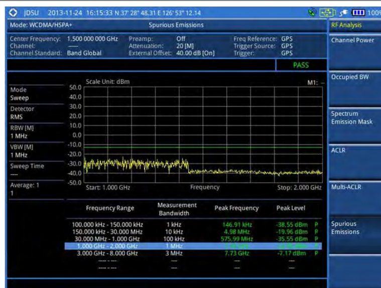
Figure 63 Spurious emissions measurement with WCDMA/HSPA+ signal analyzer
