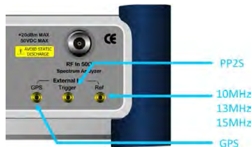
Figure 81 Connection ports for external reference clock
