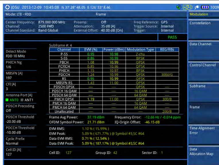
Figure 99 Frame measurement with LTE - FDD signal analyzer (MBMS On)
