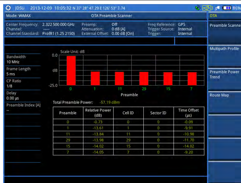
Figure 241 Preamble scanner measurement with Mobile WiMAX OTA signal analyzer
