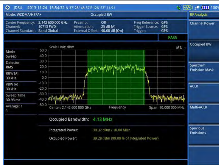
Figure 59 Occupied bandwidth measurement with WCDMA/HSPA+ signal analyzer
