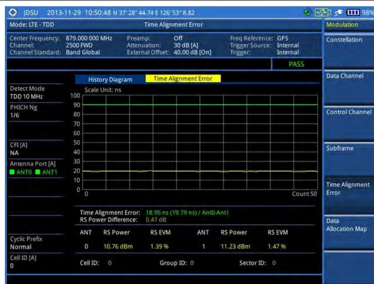
Figure 137 Time alignment error measurement with LTE - TDD signal analyzer
