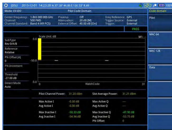
Figure 190 Code domain power measurement with EV-DO signal analyzer
