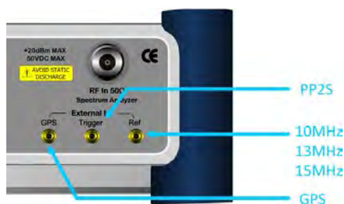
Figure 56 Connection ports for external reference clock
