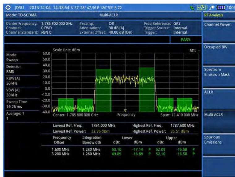
Figure 210 Multi-ACLR measurement with TD-SCDMA signal analyzer
