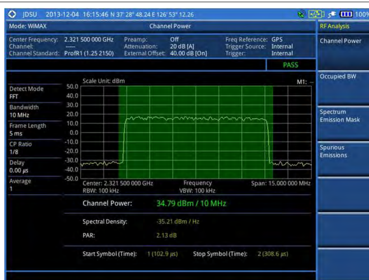
Figure 231 Channel power measurement with Mobile WiMAX signal analyzer
