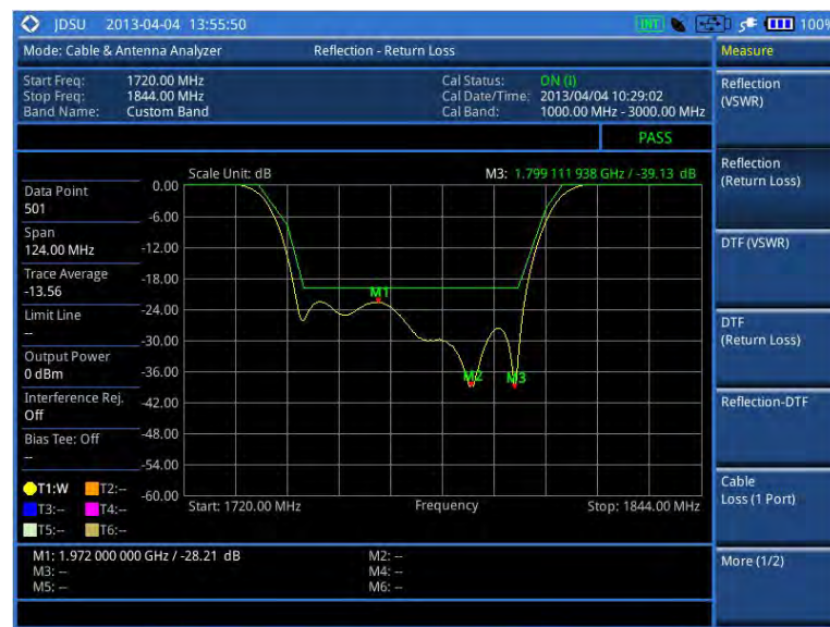
Figure 255 Reflection measurement in return loss scale
