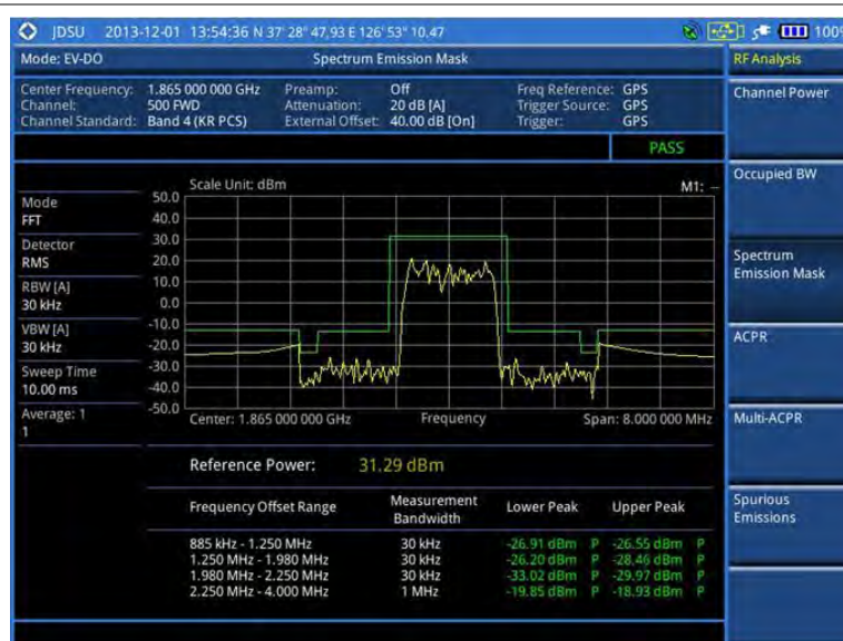
Figure 183 SEM measurement with EV-DO signal analyzer
