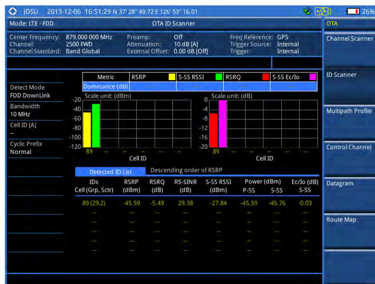
Figure 108 ID scanner measurement with LTE - FDD OTA signal analyzer
