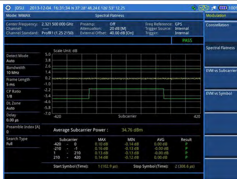
Figure 237 Spectral flatness measurement with Mobile WiMAX signal analyzer
