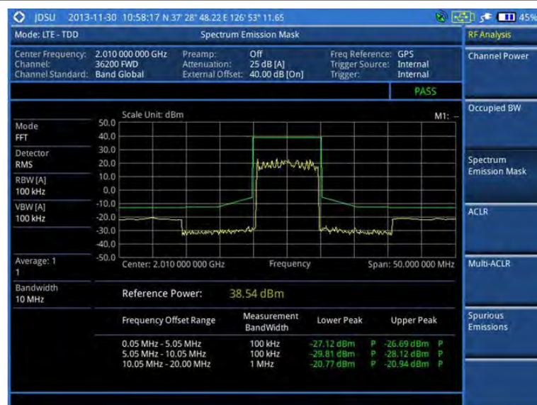
Figure 123 SEM measurement with LTE - TDD signal analyzer
