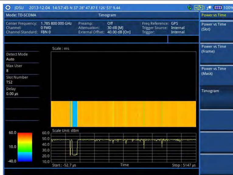
Figure 215 Timogram with TD-SCDMA signal analyzer
