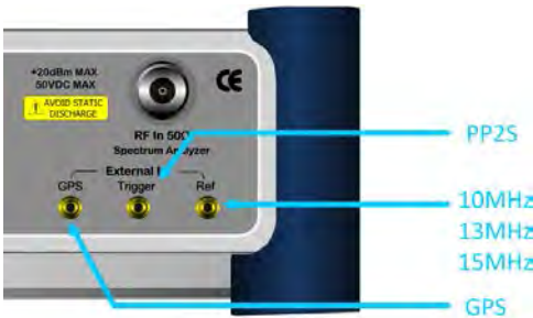
Figure 204 Connection ports for external reference clock
