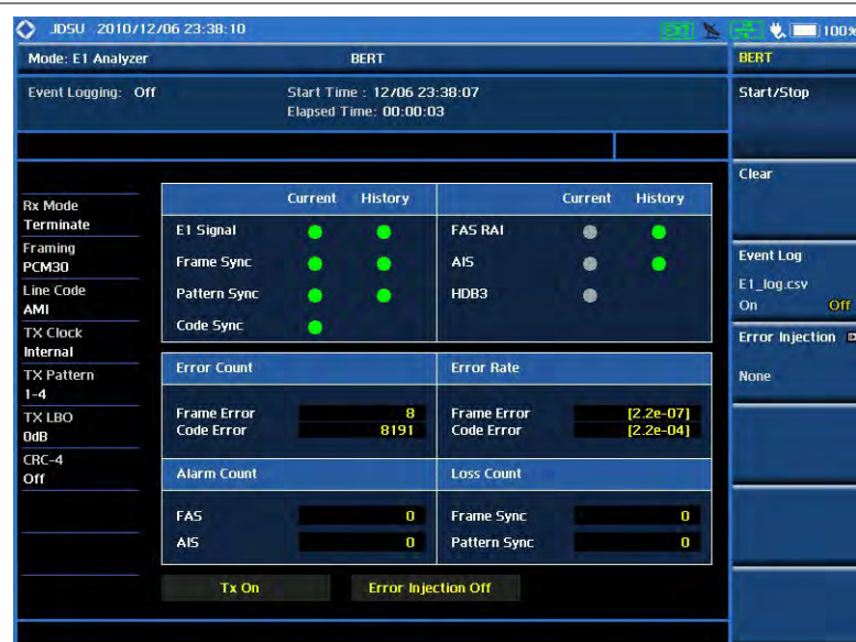
Figure 272 E1 BERT testing for framing PCM30
