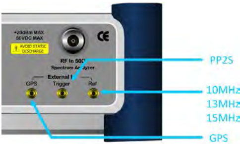
Figure 156 Connection ports for external reference clock
