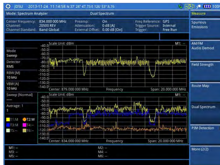
Figure 21 Dual spectrum measurement with spectrum analyzer
