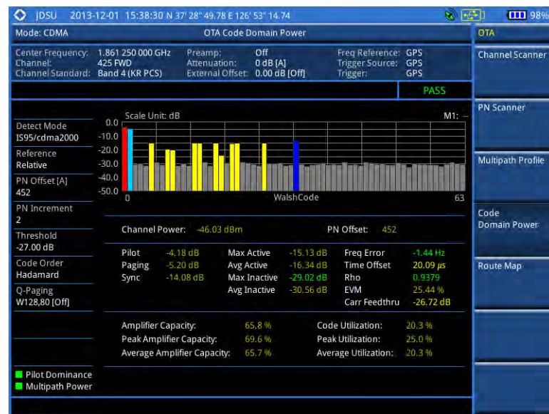
Figure 173 Code domain power measurement with CDMA OTA signal analyzer
