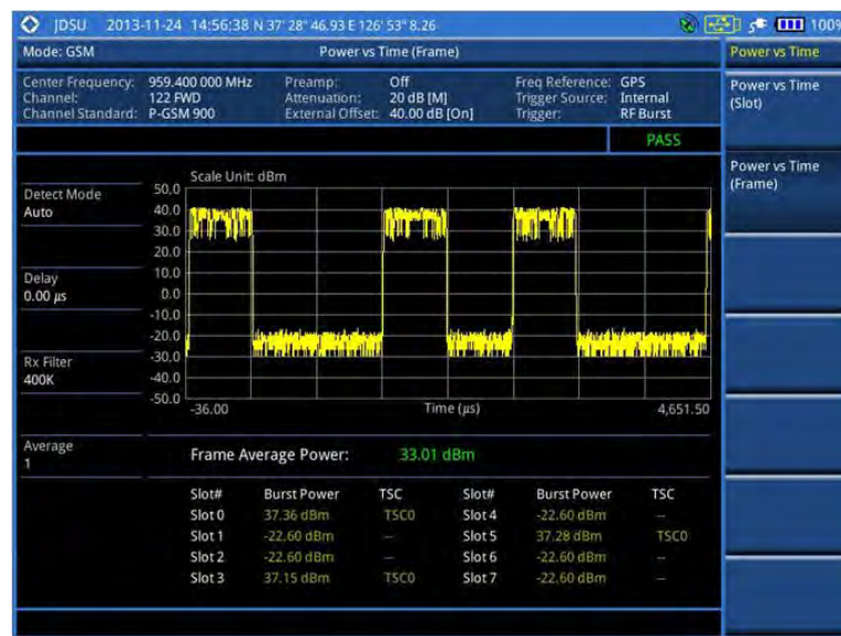
Figure 46 Power vs. time (frame) measurement with GSM signal analyzer
