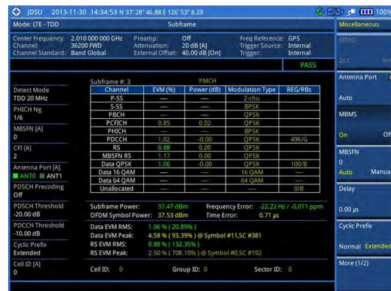
Figure 136 Subframe measurement with LTE - TDD signal analyzer (MBMS On)
