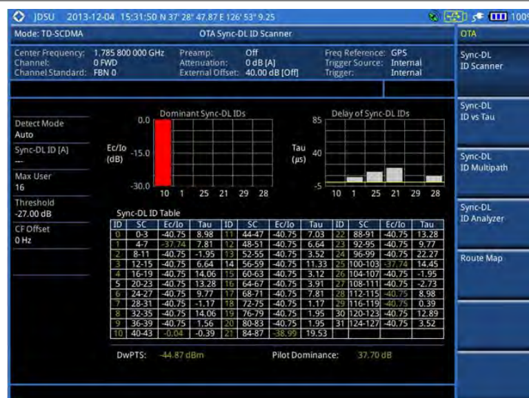
Figure 220 Sync-DL ID scanner measurement with TD-SCDMA OTA signal analyzer
