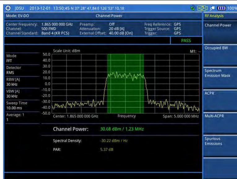
Figure 181 Channel power measurement with EV-DO signal analyzer
