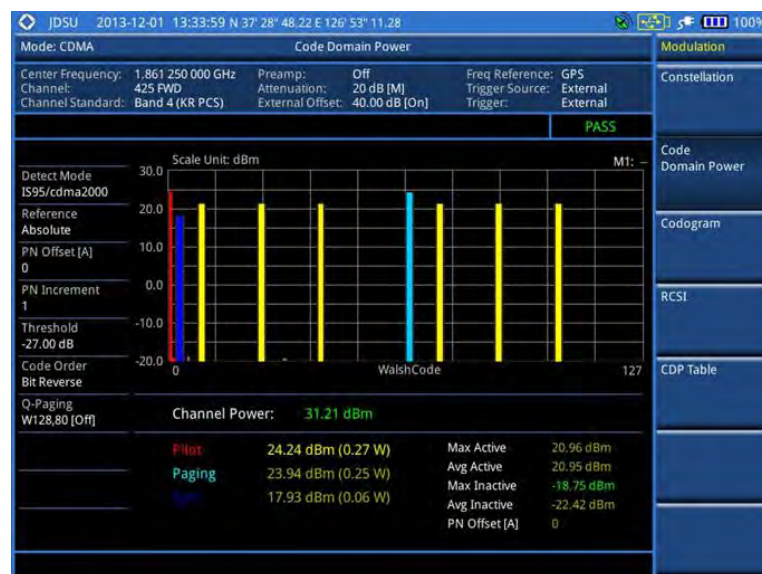
Figure 165 Code domain power measurement with CDMA signal analyzer
