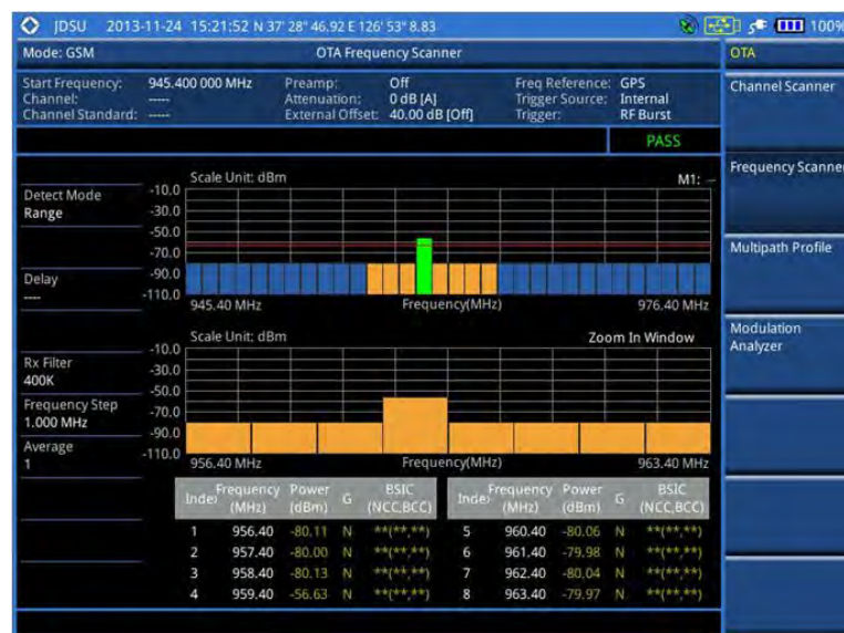
Figure 49 Frequency scanner measurement with GSM OTA signal analyzer
