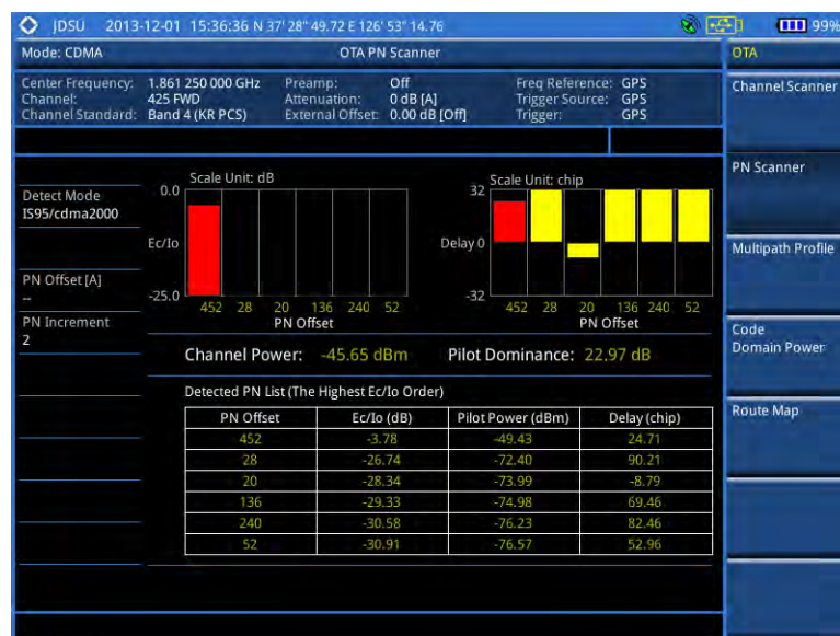
Figure 171 PN scanner measurement with CDMA OTA signal analyzer
