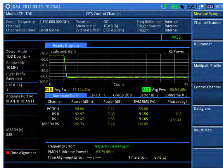
Figure 147 Control channel measurement with LTE - TDD OTA signal analyzer
