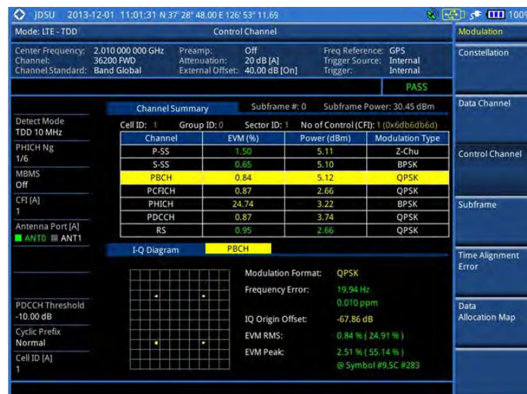
Figure 133 Control channel measurement with LTE - TDD signal analyzer
