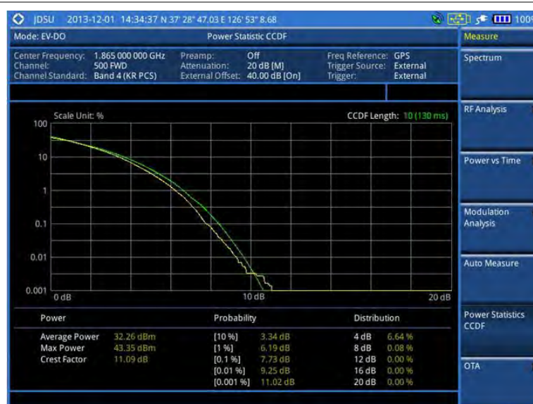
Figure 194 CCDF measurement with EV-DO signal analyzer
