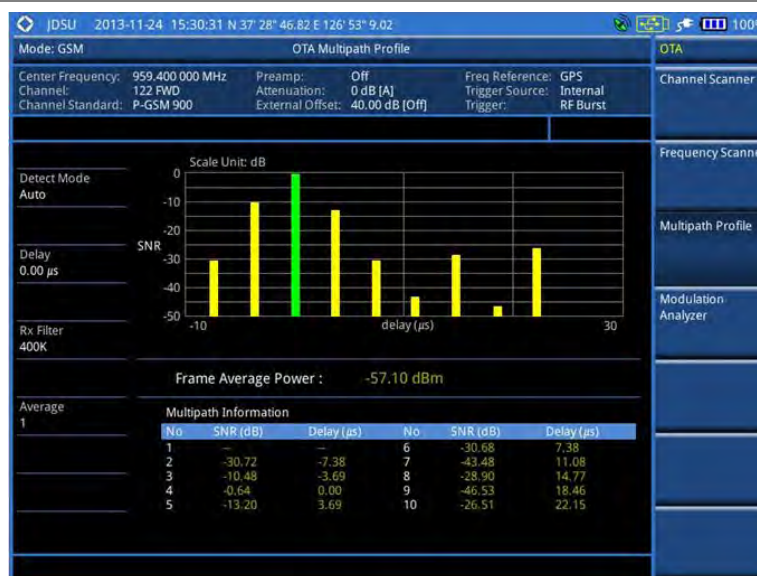
Figure 50 Multipath profile measurement with GSM OTA signal analyzer
