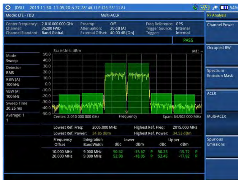
Figure 125 Multi-ACLR measurement with LTE - TDD signal analyzer
