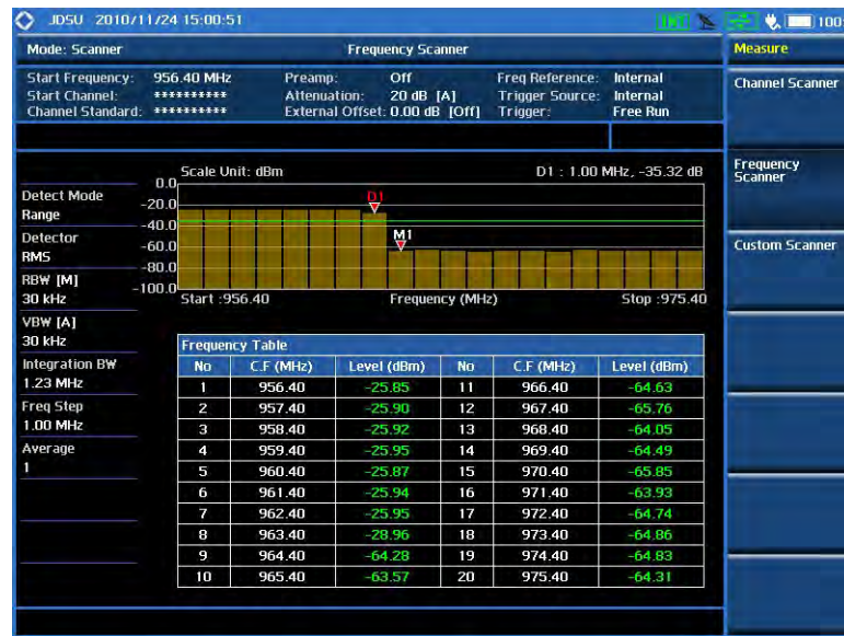
Figure 287 Frequency scanner measurement
