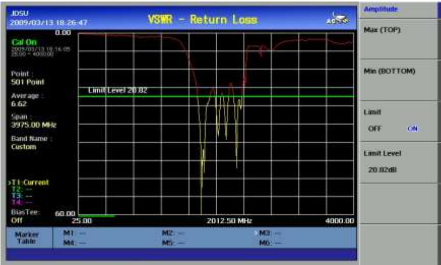
Figure 12 – Limit Line Application
