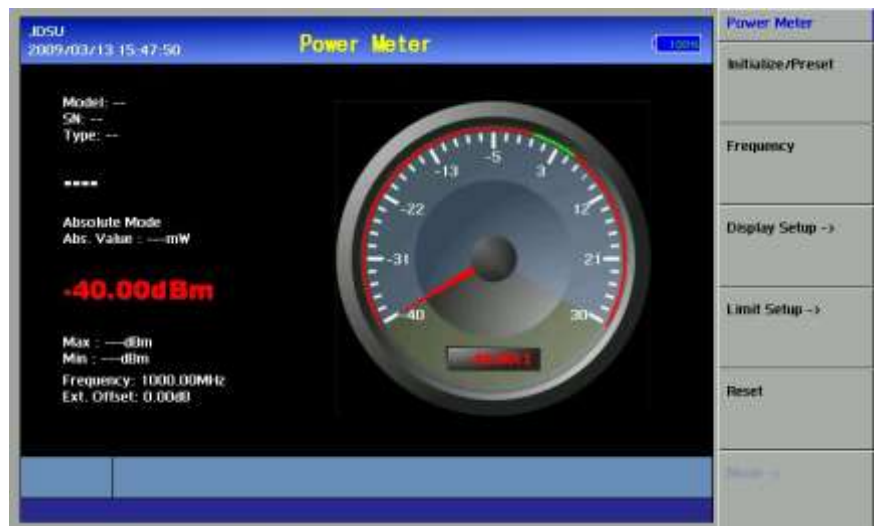
Figure 34 – Power Meter Screen before Connecting Sensor
