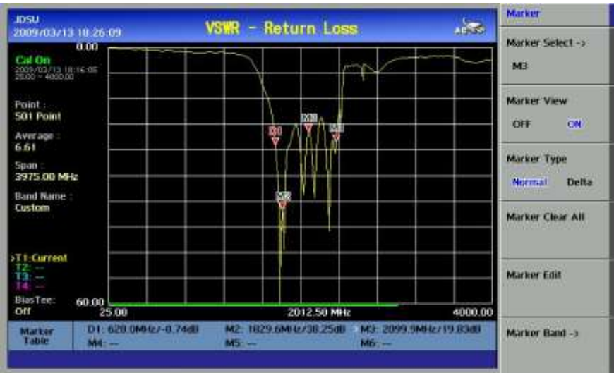
Figure 11 – Using Markers in VSWR Measurement Mode
