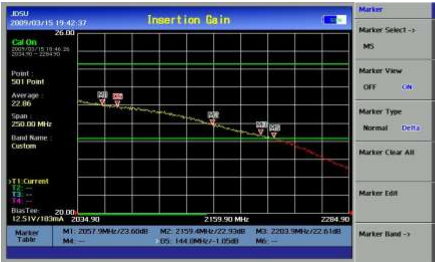
Figure 30 – Using Markers in Insertion Gain Measurement Mode
