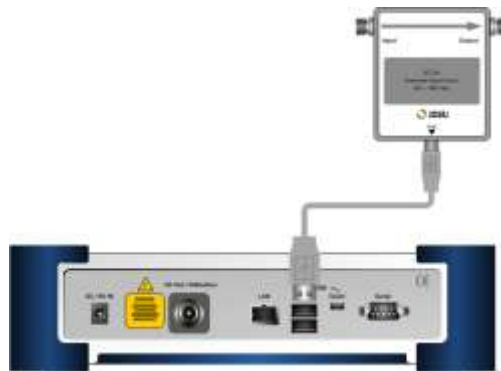
Figure 67 Cable connection diagram for directional power sensor
