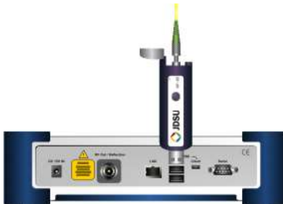
Figure 73 Cable connection diagram for optical power meter
