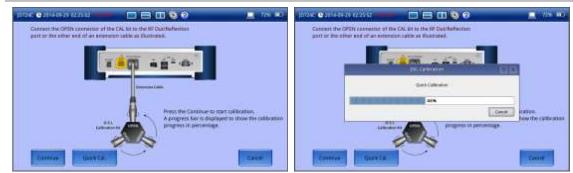
Figure 12 Quick calibration on JD724C
