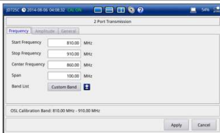
Figure 51 Frequency setup window for 2-port transmission measurements
