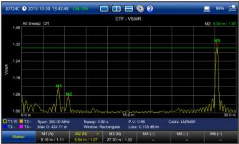
Figure 29 DTF return loss measurement screen (single layout)
