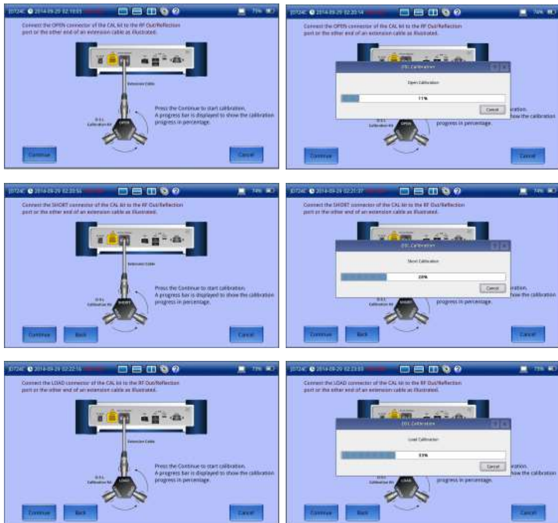
Figure 7 O-S-L calibration on JD724C using Y-Cal kit
