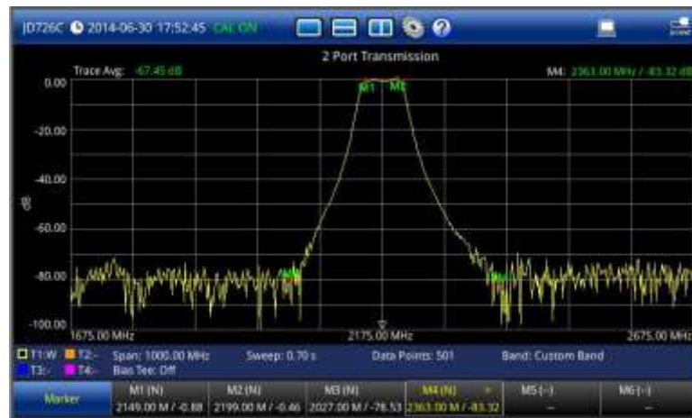
Figure 55 2 port transmission measurement screen (single layout)
