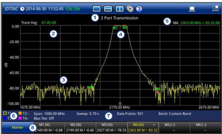
Figure 50 2 port transmission measurement screen
