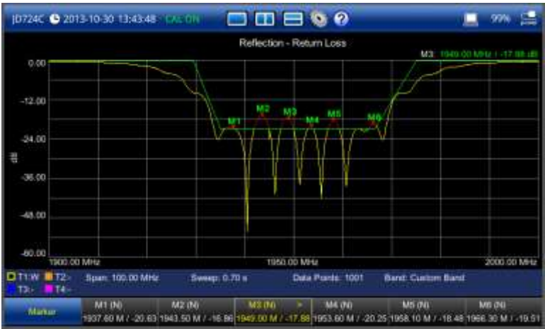
Figure 21 Reflection return loss measurement screen (zoom zones)
