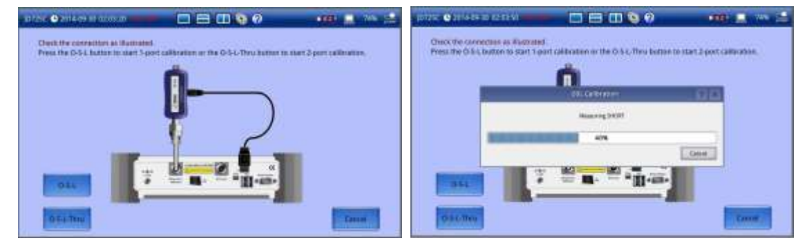
Figure 11 e-Calibration on JD725C using EZ-Cal kit
