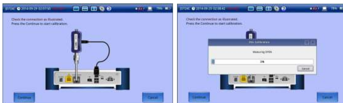
Figure 10 e-Calibration on JD724C using EZ-Cal kit
