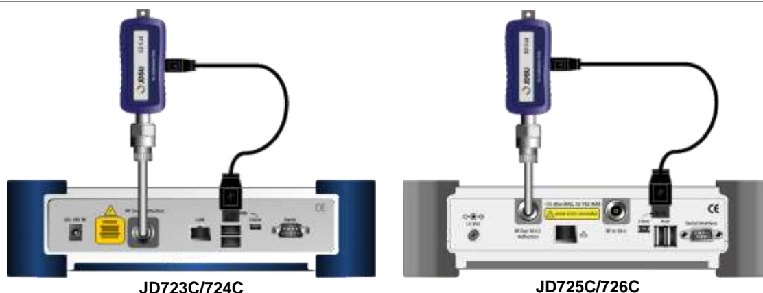
Figure 9 e-Calibration connection diagram with an extension cable
