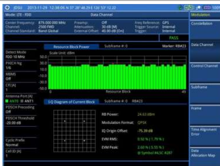
Figure 101 Data channel measurement with LTE-FDD signal analyzer
