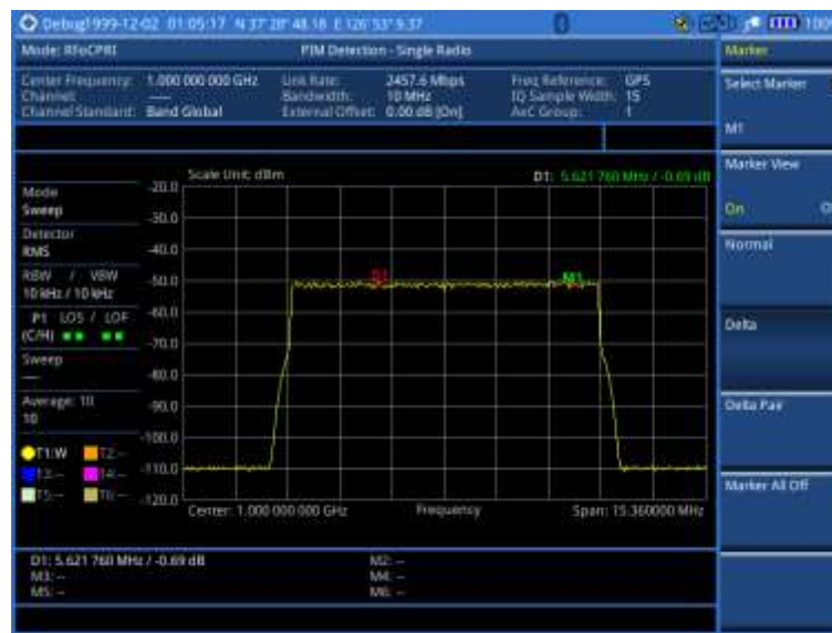
Figure 310 PIM detection of single radio
