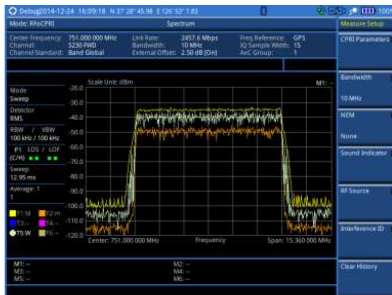
Figure 298 RFoCPRI spectrum analysis on LTE Uplink 10 MHz, antenna 1
