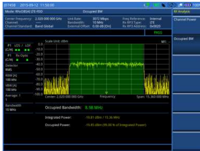
Figure 371 Occupied bandwidth measurement with RFoBSAI LTE-FDD signal analyzer
