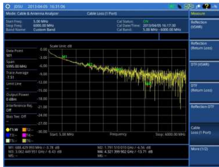
Figure 284 Cable loss (1 port) measurement
