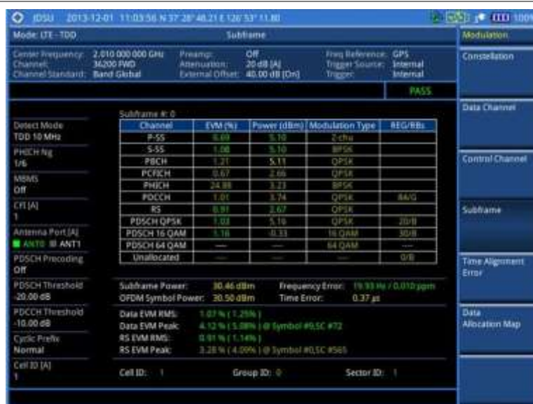
Figure 151 Subframe measurement with LTE-TDD signal analyzer
