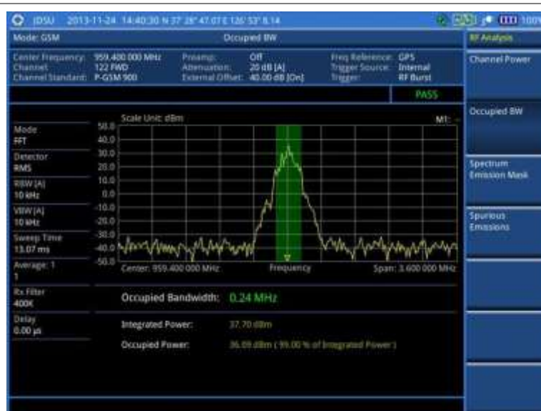
Figure 47 Occupied bandwidth measurement with GSM signal analyzer
