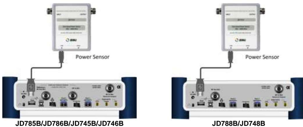
Figure 392 Directional power sensor connection
