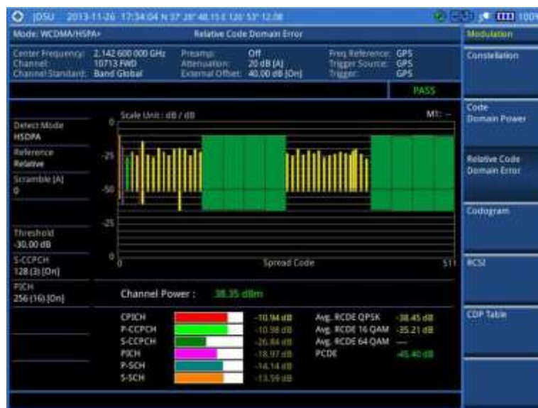
Figure 74 Relative code domain error with WCDMA/HSPA+ signal analyzer
