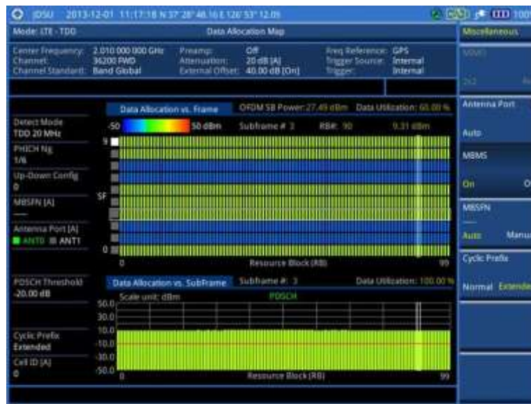
Figure 156 Data allocation map measurement with LTE-TDD signal analyzer (MBMS On)
