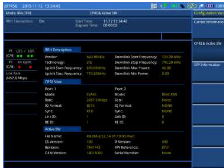
Figure 344 Example of verification of CPRI state and active software
