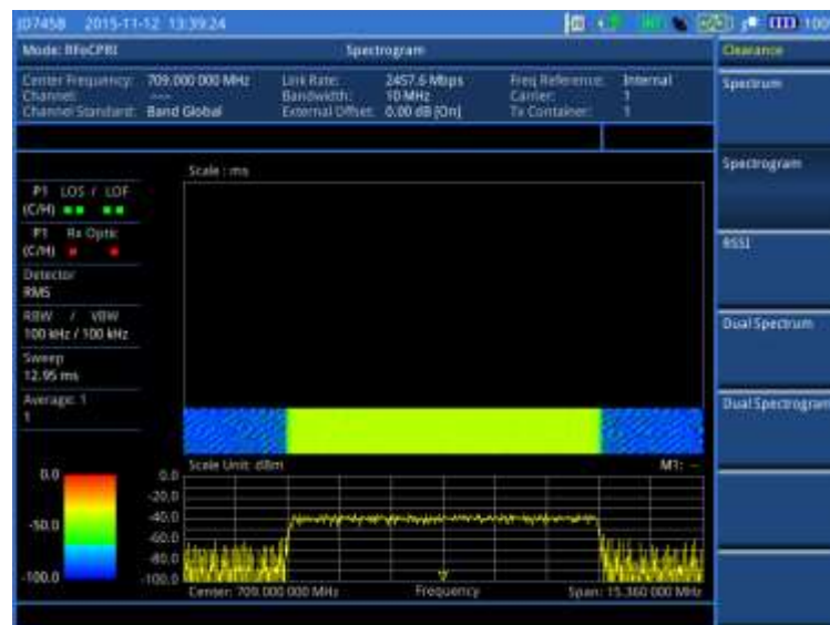
Figure 350 Example of spectrogram in BBU emulation
