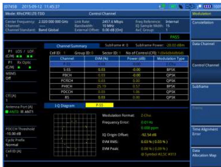
Figure 332 Control channel measurement with RFoCPRI LTE-TDD signal analyzer
