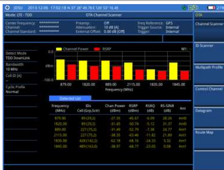
Figure 161 Channel scanner measurement with LTE-TDD OTA signal analyzer
