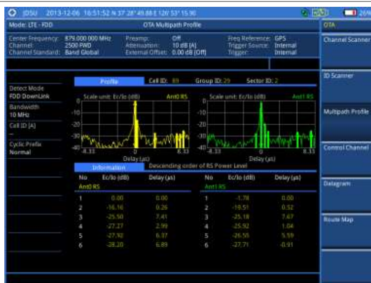
Figure 119 Multipath profile measurement with LTE-FDD OTA signal analyzer
