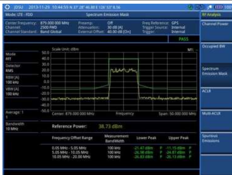
Figure 94 SEM measurement with LTE-FDD signal analyzer
