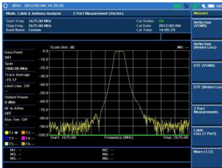
Figure 287 2-port vector measurement
