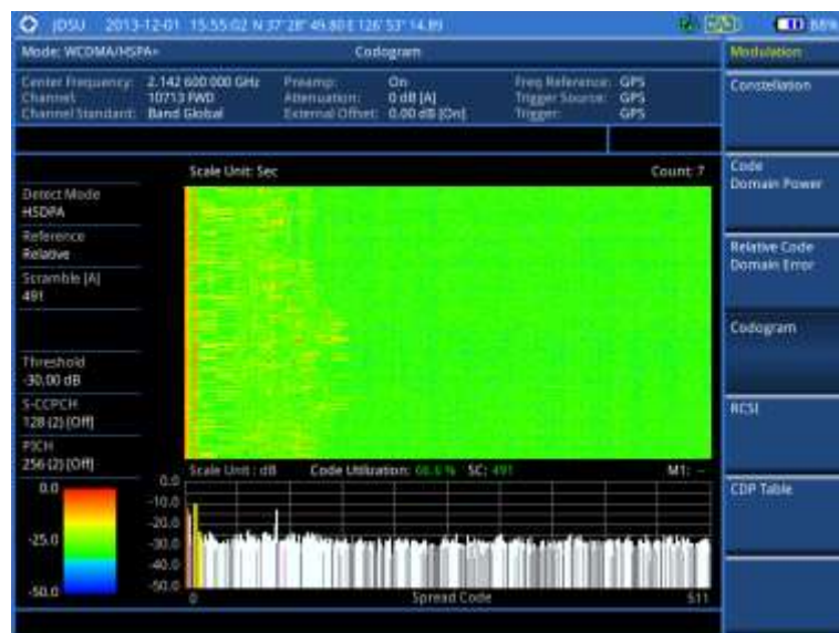
Figure 75 Codogram in full view with WCDMA/HSPA+ signal analyzer
