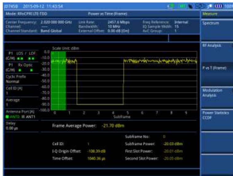
Figure 329 Power vs. time (frame) measurement with RFoCPRI LTE-TDD signal analyzer
