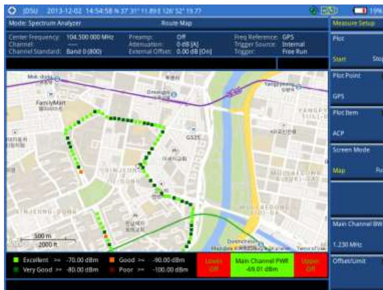
Figure 24 Route map measurement screen with GPS
