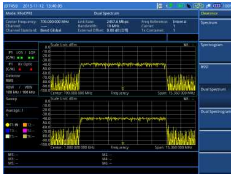
Figure 349 Example of dual spectrum analysis in BBU emulation
