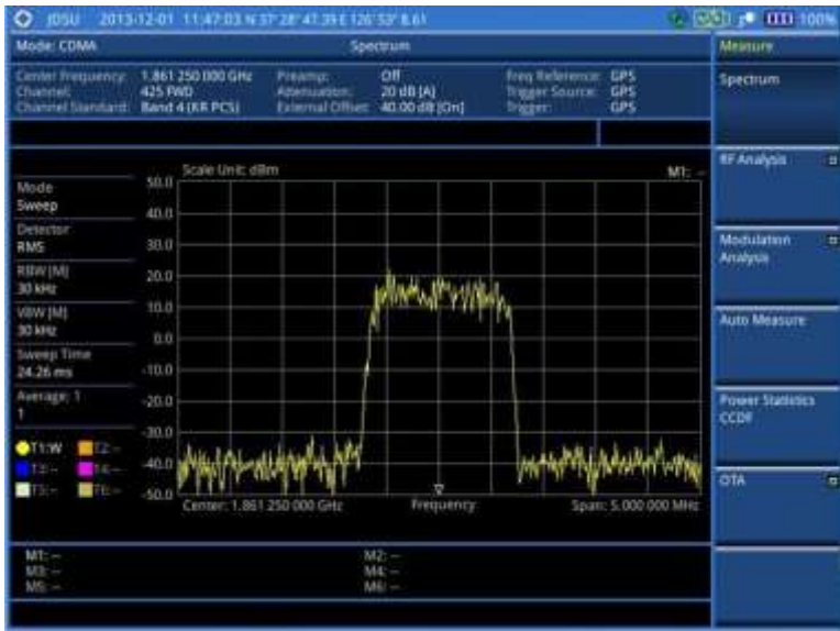
Figure 180 Spectrum measurement screen with CDMA signal analyzer
