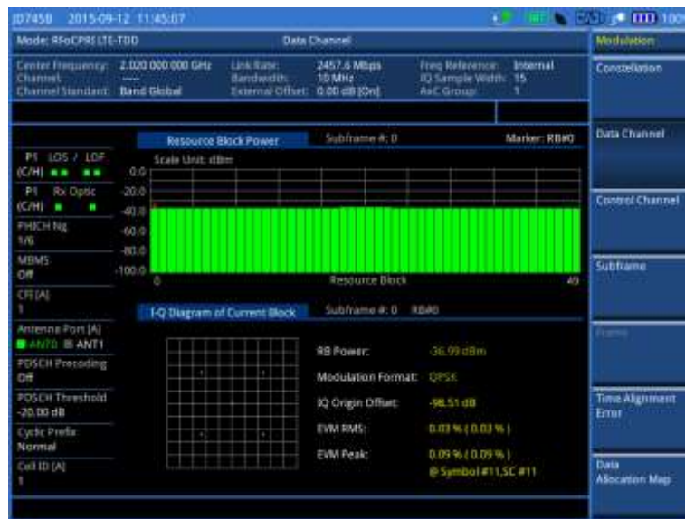
Figure 331 Data channel measurement with RFoCPRI LTE-FDD signal analyzer
