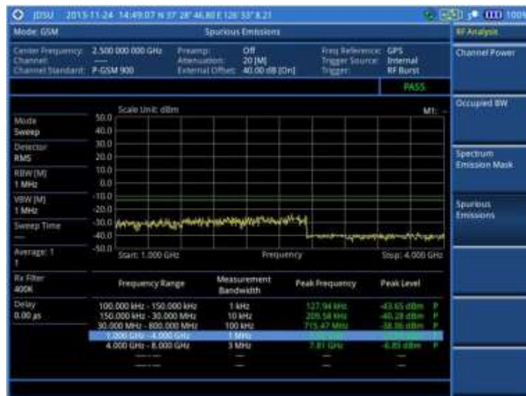
Figure 50 Spurious emissions measurement with GSM signal analyzer
