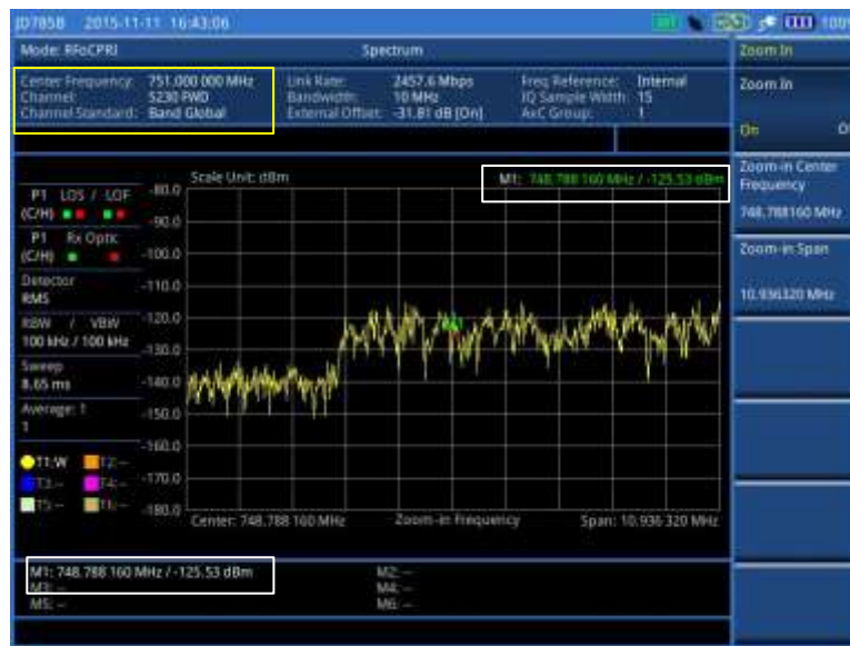
Figure 307 Zoomed-in spectrum view in RFoCPRI interference analyzer
