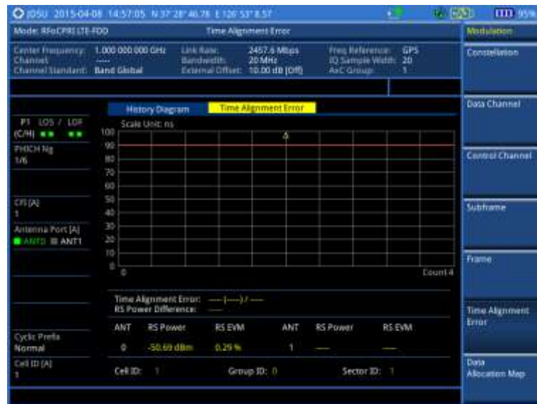
Figure 322 Time alignment error measurement with RFoCPRI LTE-FDD signal analyzer
