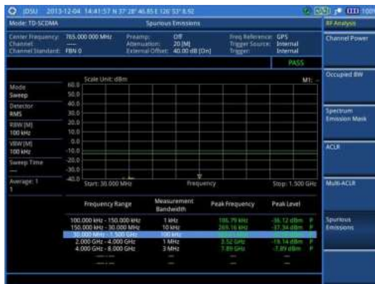
Figure 234 Spurious emissions measurement with TD-SCDMA signal analyzer
