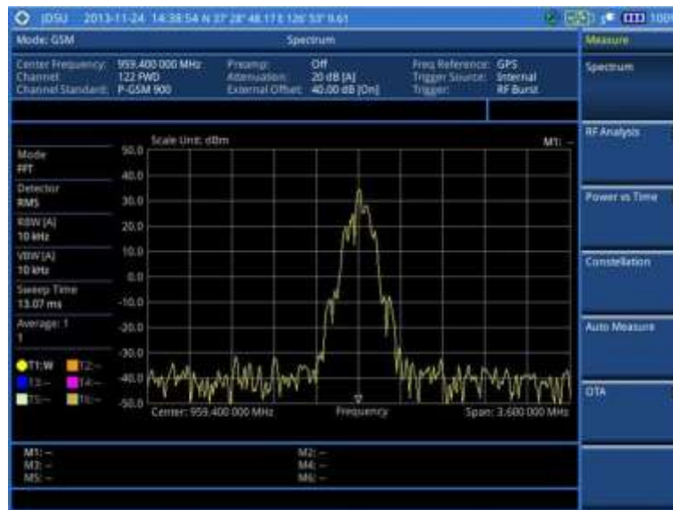
Figure 45 Spectrum measurement screen with GSM signal analyzer
