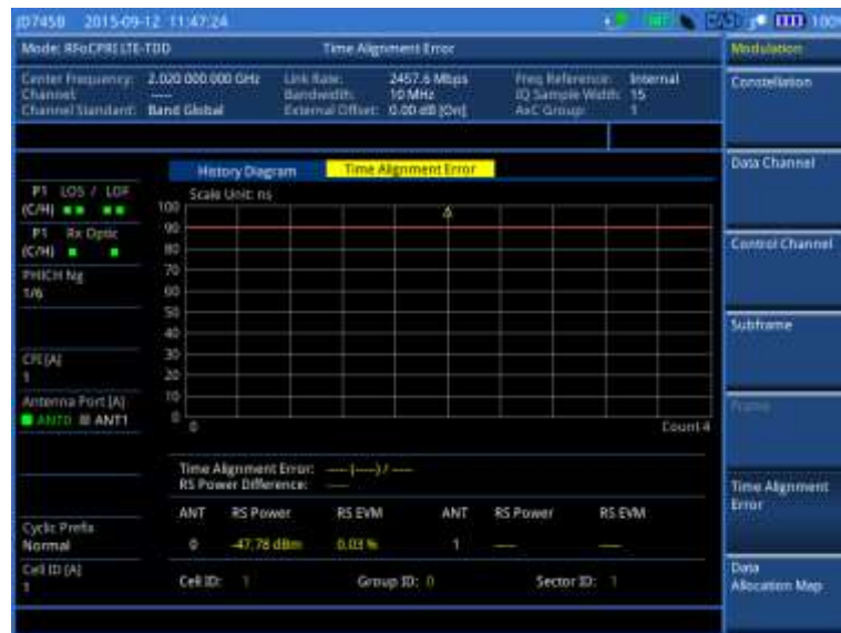
Figure 334 Time alignment error measurement with RFoCPRI LTE-TDD signal analyzer
