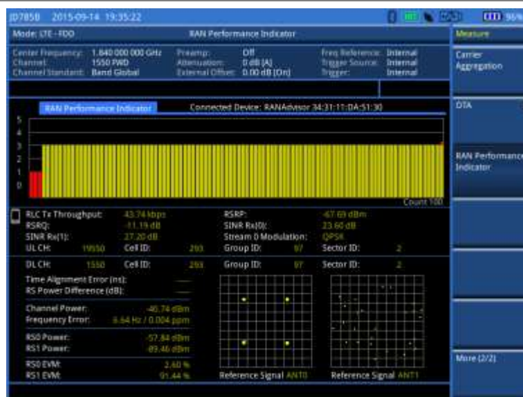
Figure 130 RAN performance indicator with LTE-FDD signal analyzer
