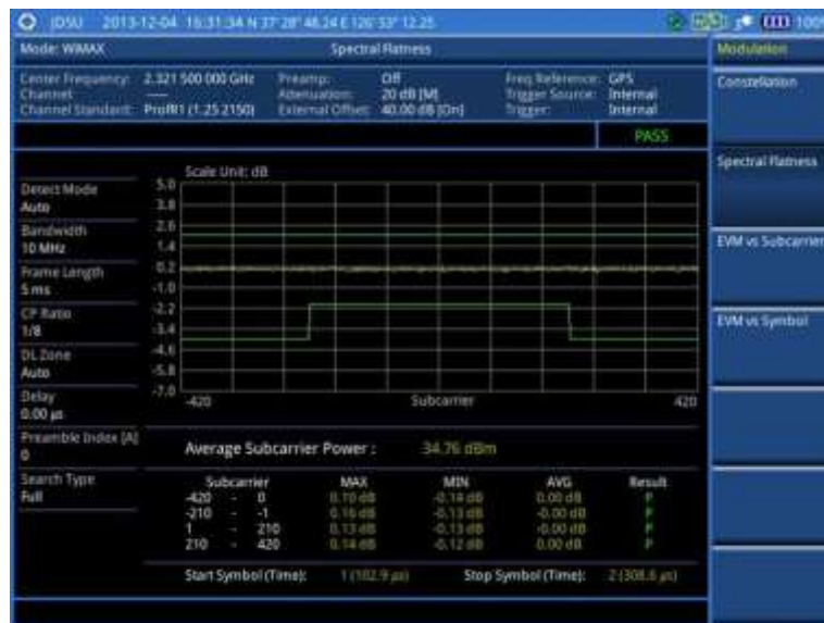
Figure 260 Spectral flatness measurement with Mobile WiMAX signal analyzer
