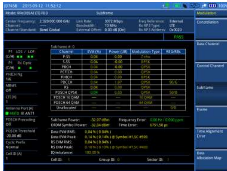
Figure 376 Subframe measurement with RFoBSAI LTE-FDD signal analyzer
