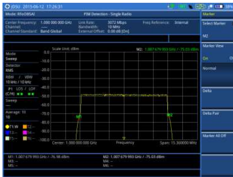
Figure 367 PIM detection of single radio
