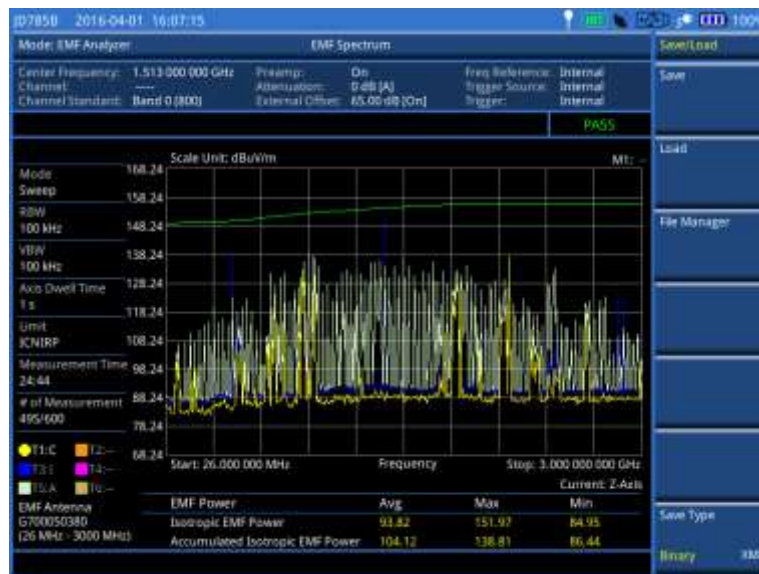
Figure 402 EMF spectrum measurement with EMF analyzer
