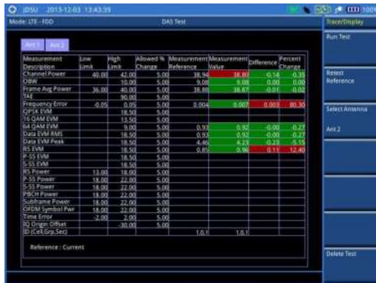
Figure 113 DAS measurement with LTE-FDD signal analyzer
