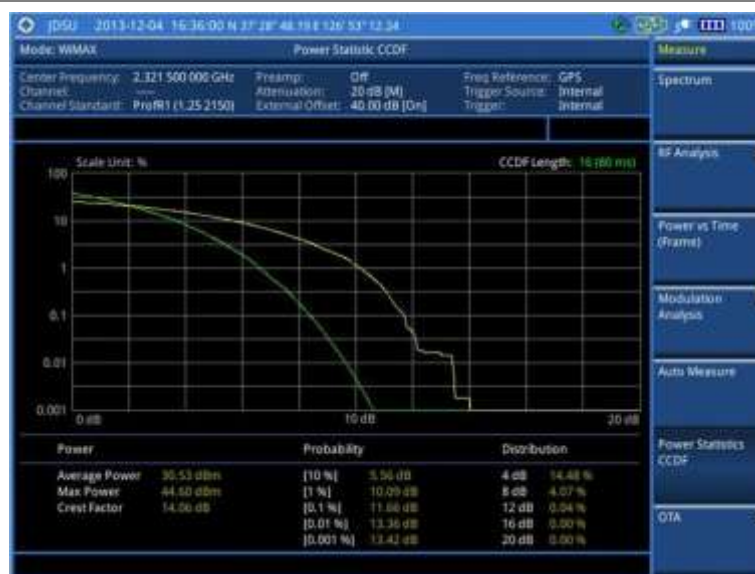
Figure 263 CCDF measurement with Mobile WiMAX signal analyzer
