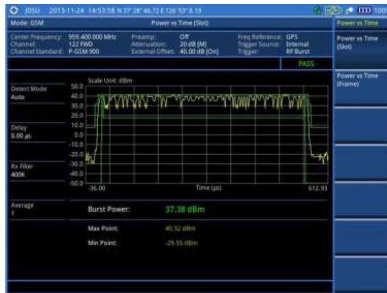
Figure 52 Power vs. time (slot) measurement with GSM signal analyzer
