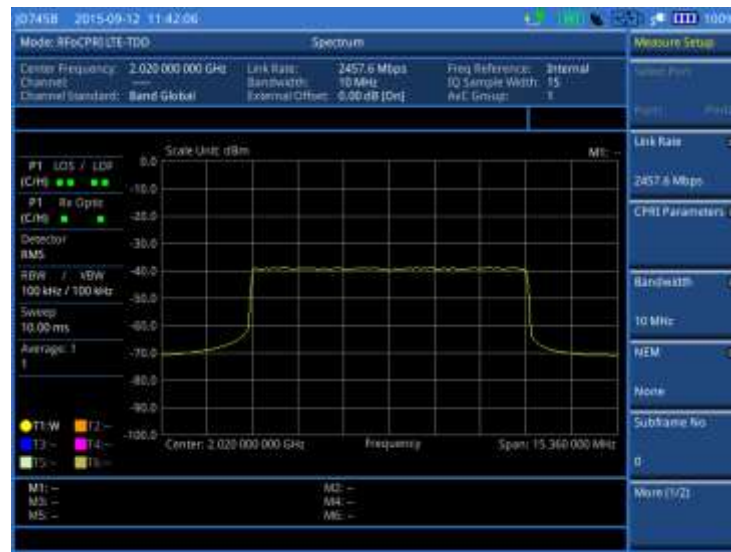
Figure 326 Spectrum measurement with RFoCPRI LTE-TDD signal analyzer
