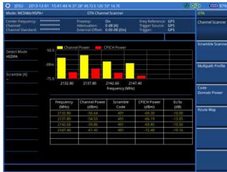
Figure 79 Channel scanner measurement with WCDMA/HSPA+ OTA signal analyzer
