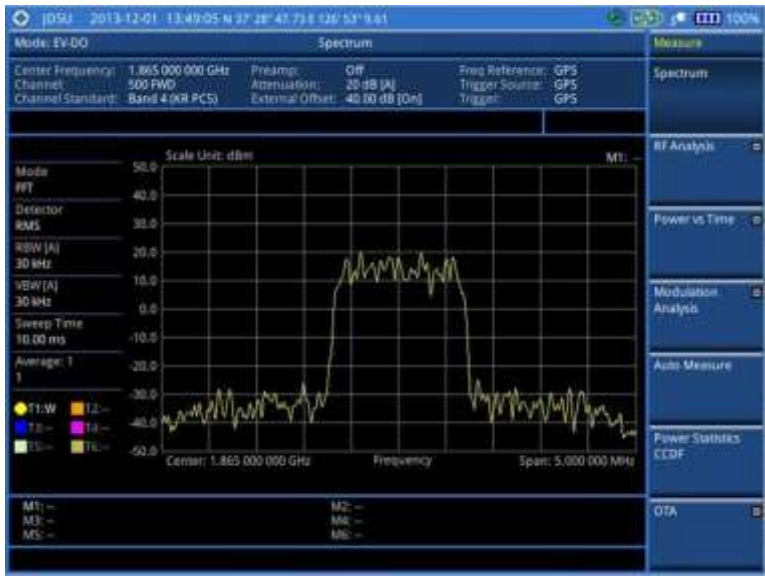
Figure 203 Spectrum measurement screen with EV-DO signal analyzer
