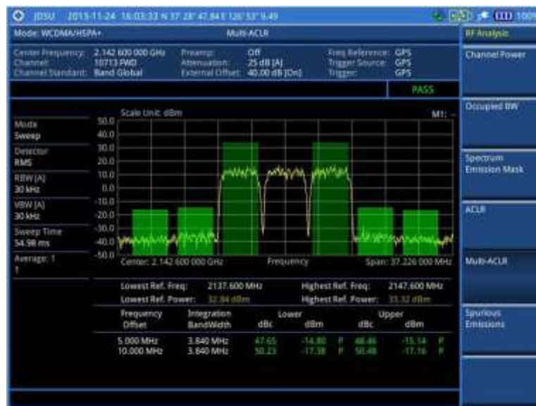
Figure 70 Multi-ACLR measurement with WCDMA/HSPA+ signal analyzer
