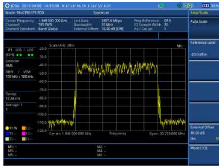
Figure 313 Spectrum measurement with RFoCPRI LTE-FDD signal analyzer
