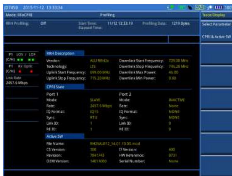
Figure 340 Example of RRH profiling results with CPRI state and activated SW
