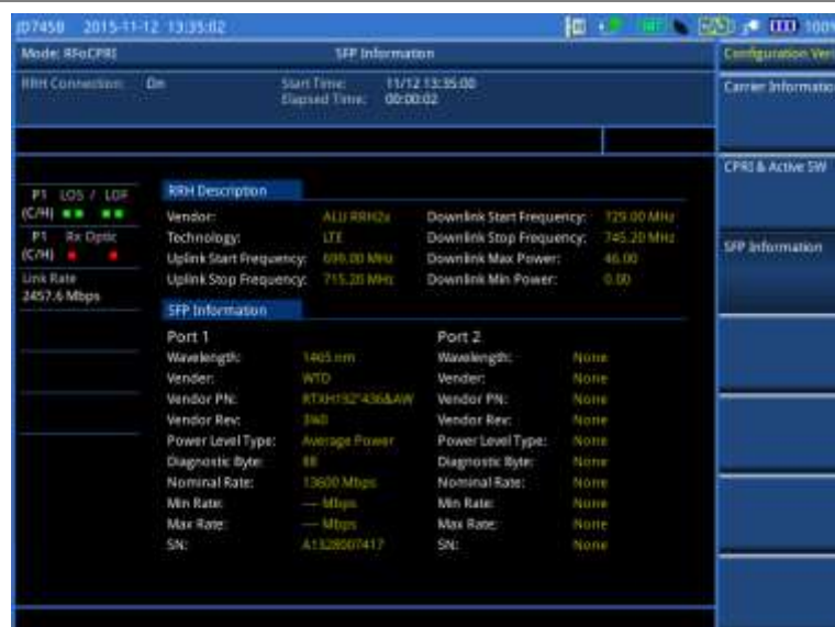
Figure 345 Example of verification of SFP information
