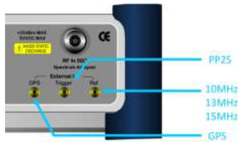
Figure 252 Connection ports for external reference clock
