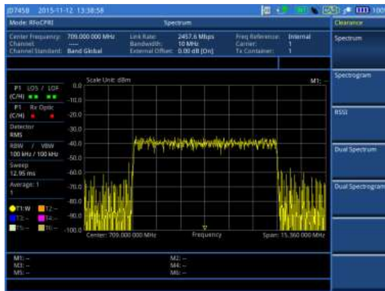
Figure 348 Example of spectrum measurement in BBU emulation
