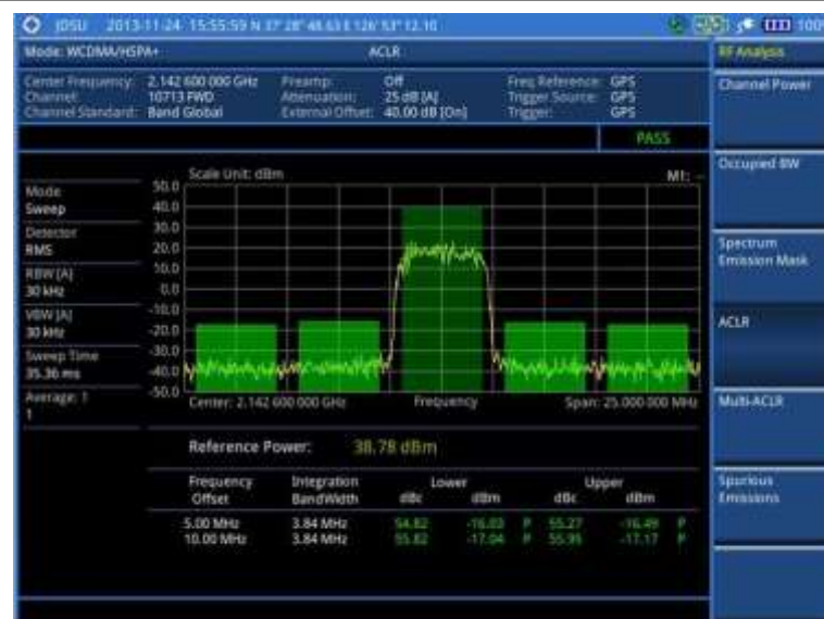
Figure 69 ACLR measurement with WCDMA/HSPA+ signal analyzer
