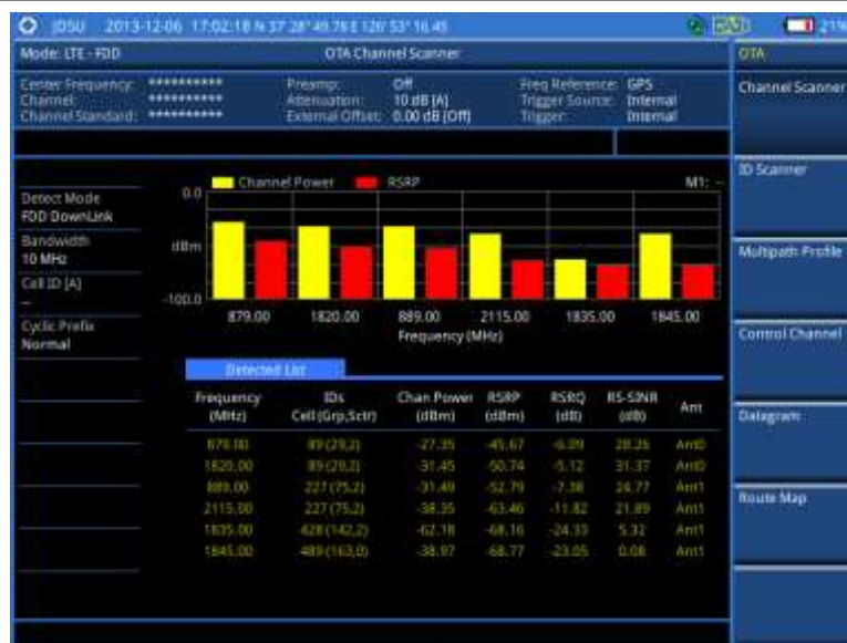
Figure 117 Channel scanner measurement with LTE-FDD OTA signal analyzer
