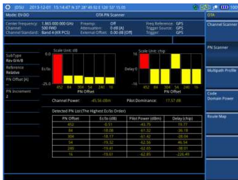
Figure 219 PN scanner measurement with EV-DO OTA signal analyzer
