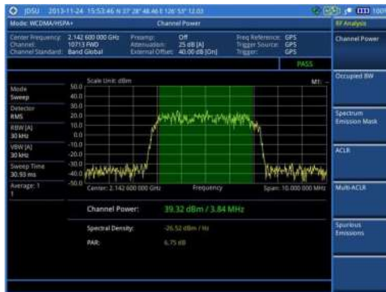
Figure 66 Channel power measurement with WCDMA/HSPA+ signal analyzer
