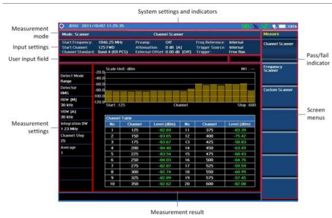
Figure 381 Channel scanner screen
