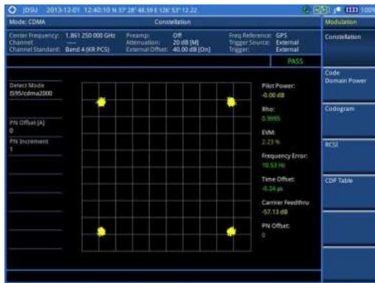
Figure 187 Constellation measurement with CDMA signal analyzer
