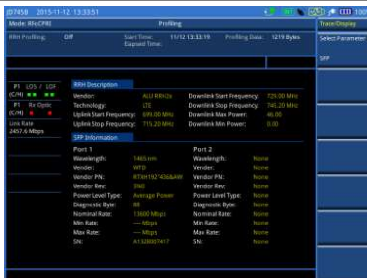
Figure 341 Example of RRH profiling results with SFP information
