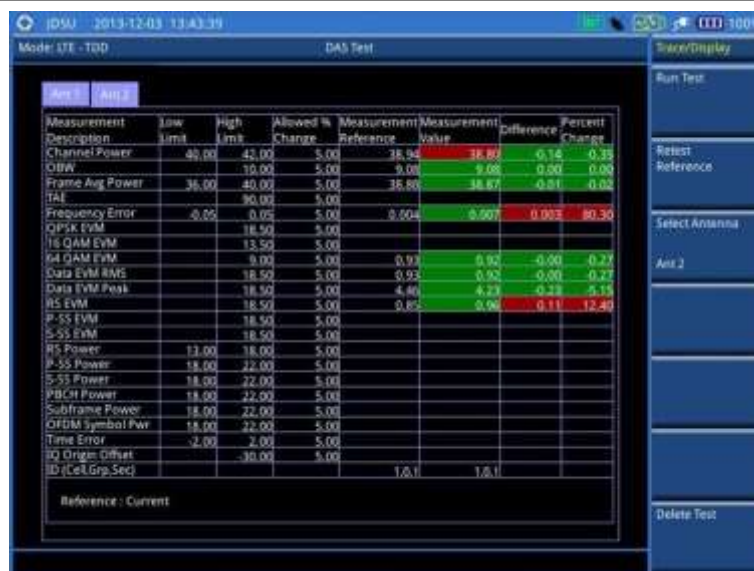
Figure 157 DAS measurement with LTE-TDD signal analyzer
