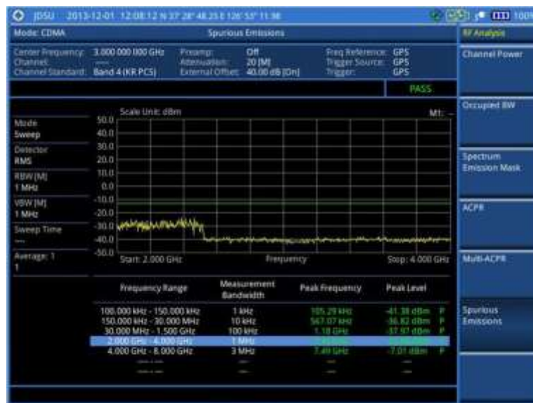
Figure 186 Spurious emissions measurement with CDMA signal analyzer
