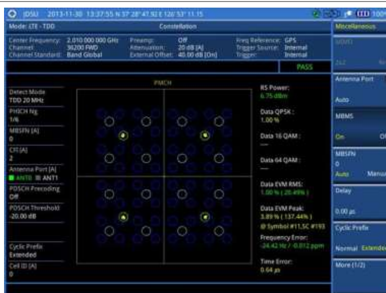
Figure 146 Constellation measurement with LTE-TDD signal analyzer (MBMS On)
