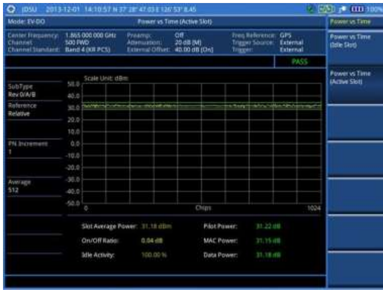
Figure 211 Power vs. time (active slot) measurement with EV-DO signal analyzer
