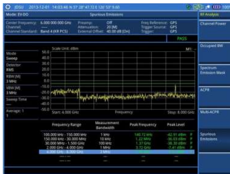
Figure 209 Spurious emissions measurement with EV-DO signal analyzer
