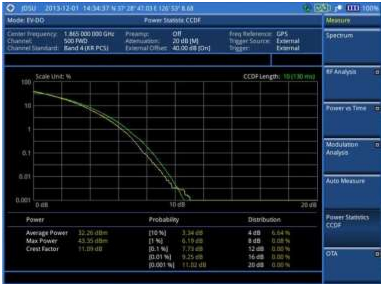
Figure 217 CCDF measurement with EV-DO signal analyzer
