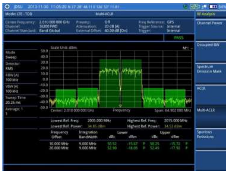
Figure 141 Multi-ACLR measurement with LTE-TDD signal analyzer
