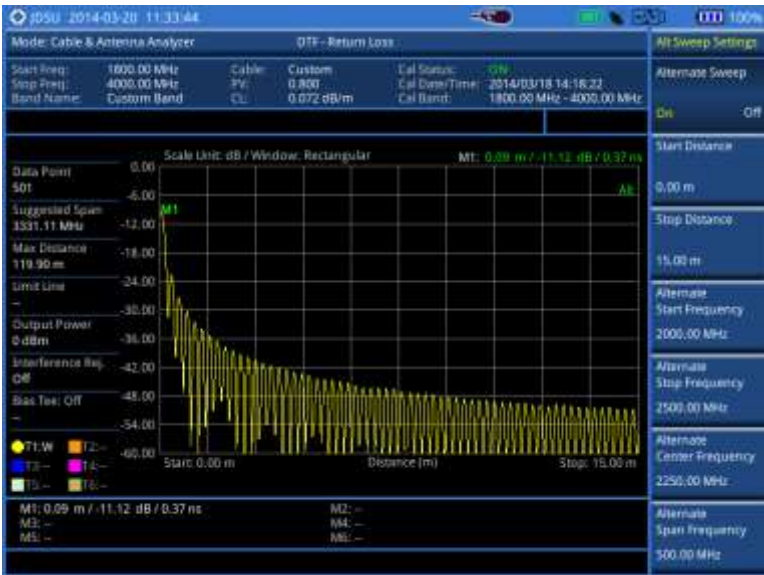
Figure 280 DTF measurement with the alternate sweep on
