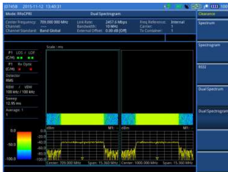
Figure 351 Example of dual spectrogram analysis in BBU emulation
