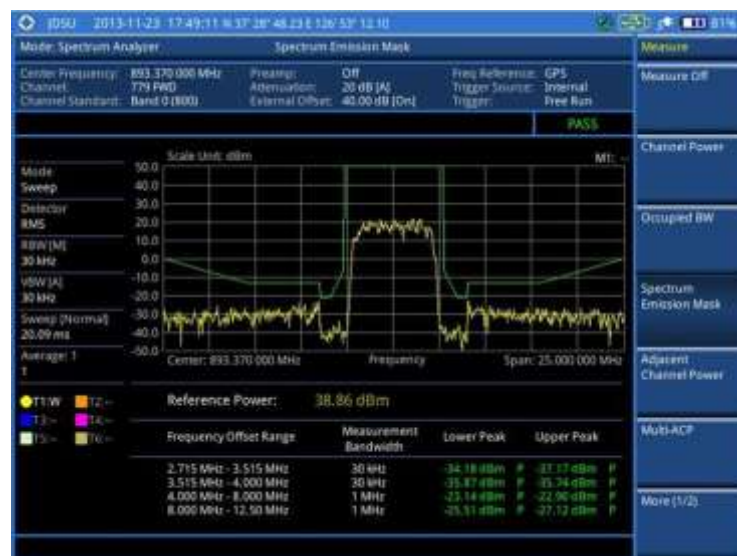
Figure 18 Spectrum emission mask measurement with spectrum analyzer
