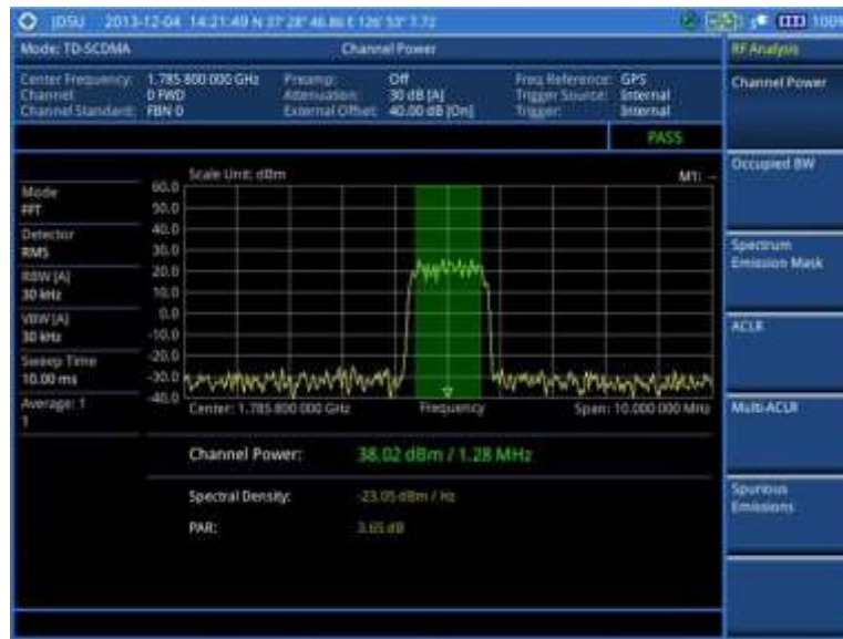
Figure 229 Channel power measurement with TD-SCDMA signal analyzer
