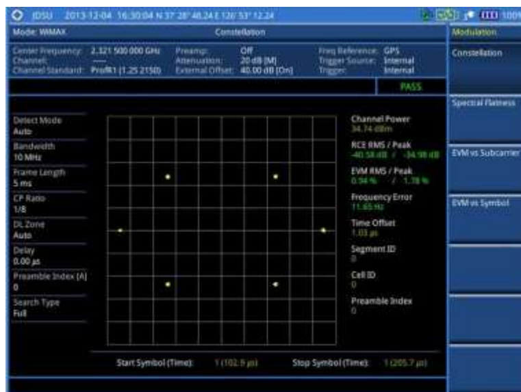
Figure 259 Constellation measurement with Mobile WiMAX signal analyzer
