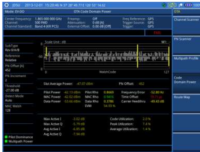
Figure 221 Code domain power measurement with EV-DO OTA signal analyzer
