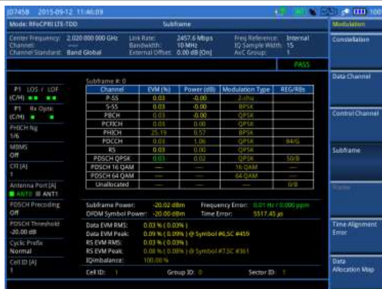
Figure 333 Subframe measurement (regular view) with RFoCPRI LTE-TDD signal analyzer
