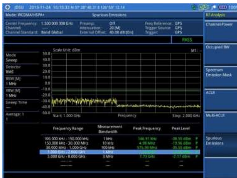
Figure 71 Spurious emissions measurement with WCDMA/HSPA+ signal analyzer
