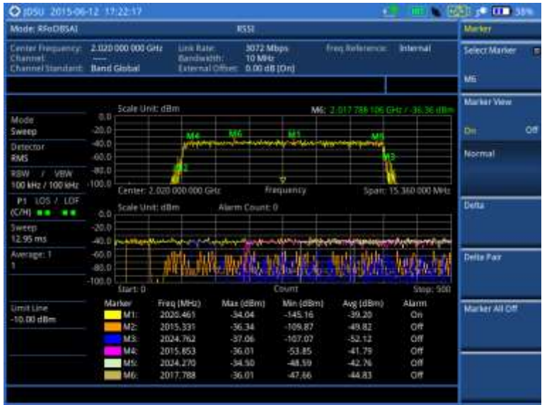
Figure 364 RFoBSAI interference measurement in RSSI
