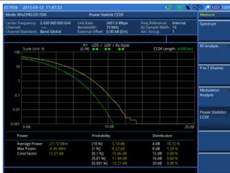
Figure 336 CCDF measurement with RFoCPRI LTE-TDD signal analyzer
