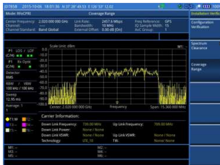
Figure 353 Example of coverage range in BBU emulation
