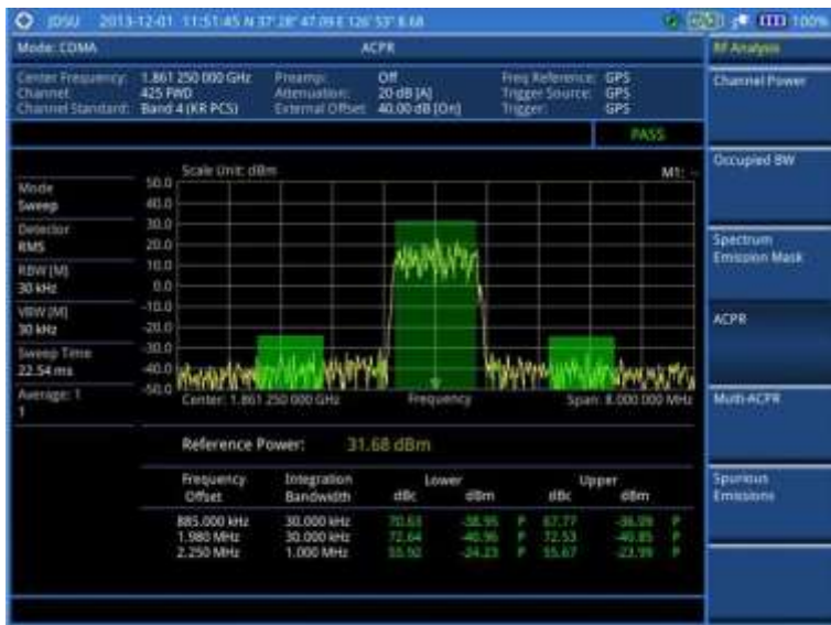
Figure 184 ACPR measurement with CDMA signal analyzer
