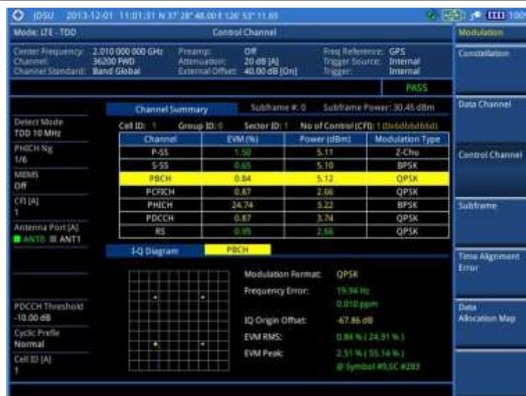
Figure 149 Control channel measurement with LTE-TDD signal analyzer
