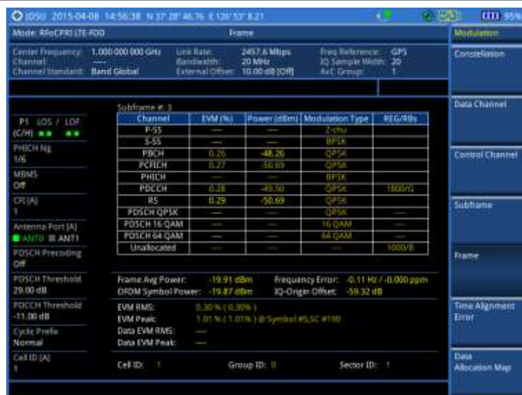
Figure 321 Frame measurement with RFoCPRI LTE-FDD signal analyzer
