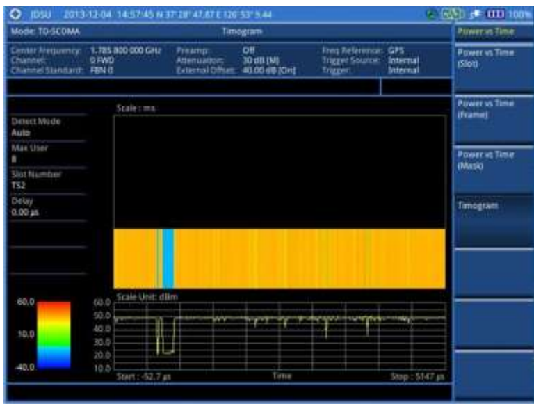
Figure 238 Timogram with TD-SCDMA signal analyzer
