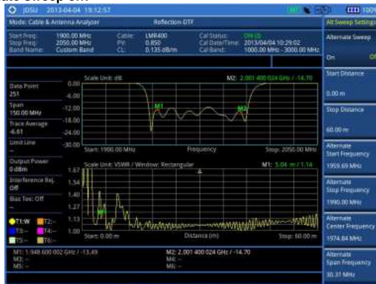
Figure 281 Reflection-DTF dual measurement
