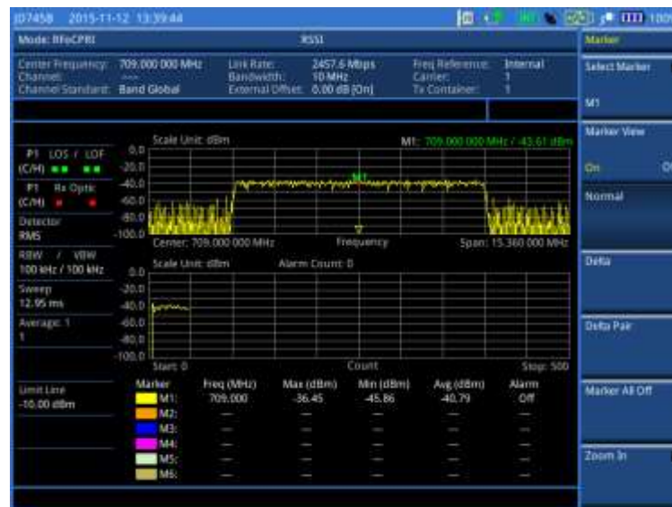
Figure 352 Example of RSSI in BBU emulation
