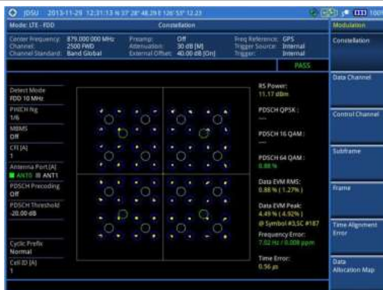
Figure 99 Constellation measurement with LTE-FDD signal analyzer
