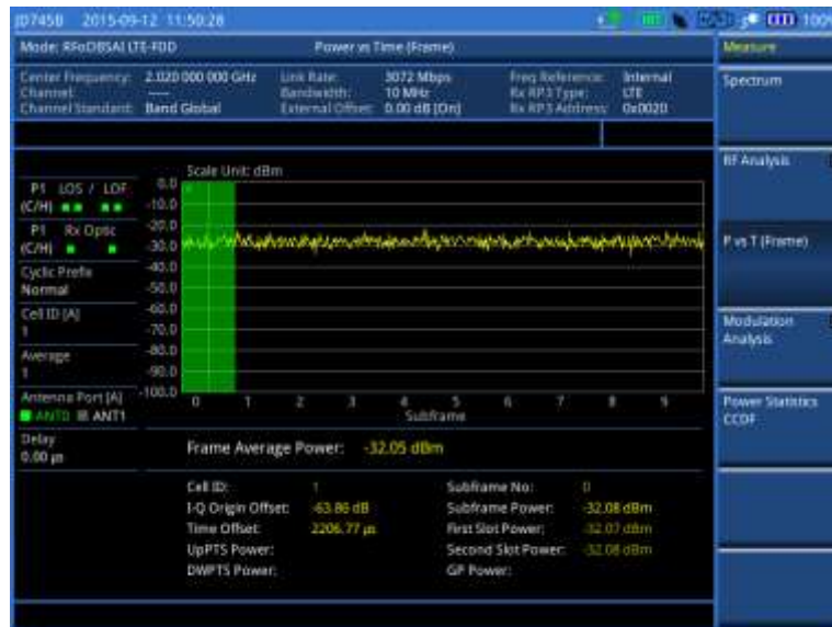
Figure 372 Power vs. time (frame) measurement with RFoOBSAI LTE-FDD signal analyzer
