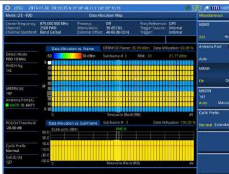
Figure 112 Data allocation map measurement with LTE-FDD signal analyzer (MBMS On)
