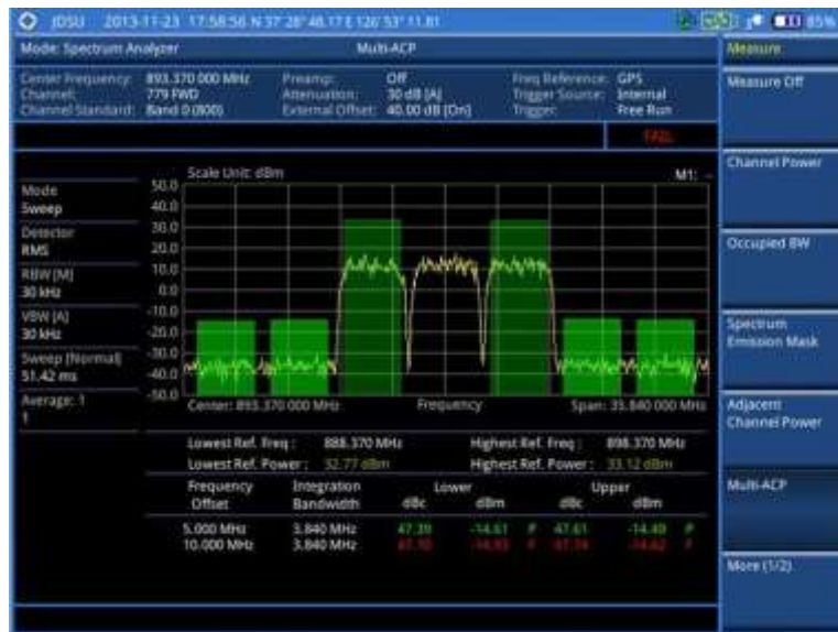
Figure 20 Multi-ACP measurement with spectrum analyzer
