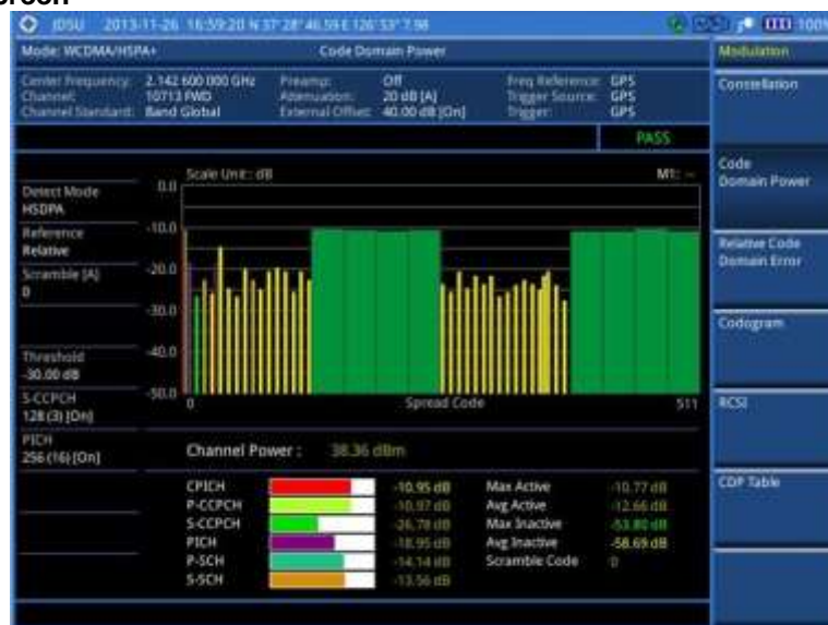
Figure 73 Code domain power measurement with WCDMA/HSPA+ signal analyzer
