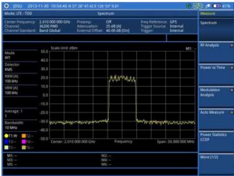
Figure 136 Spectrum measurement screen with LTE-TDD signal analyzer
