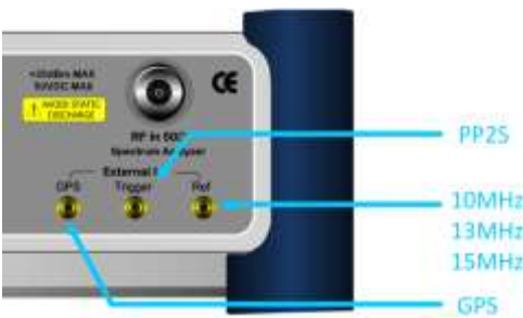
Figure 179 Connection ports for external reference clock
