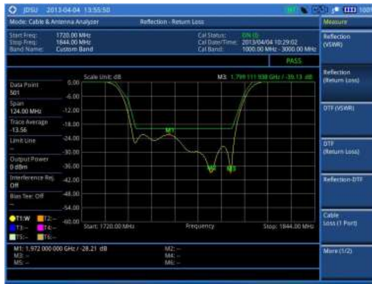
Figure 278 Reflection measurement in return loss scale
