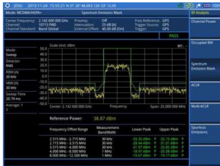
Figure 68 SEM measurement with WCDMA/HSPA+ signal analyzer
