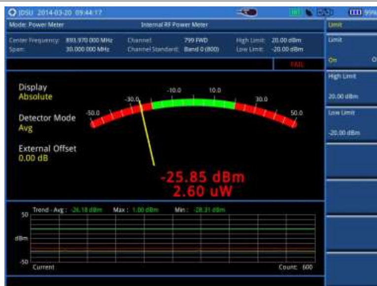
Figure 391 Internal power measurement
