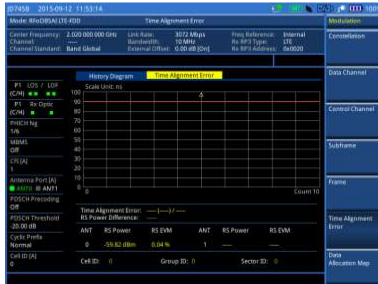
Figure 378 Time alignment error measurement with RFoBSAI LTE-FDD signal analyzer
