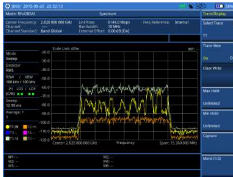
Figure 362 RFoBSAI spectrum measurement
