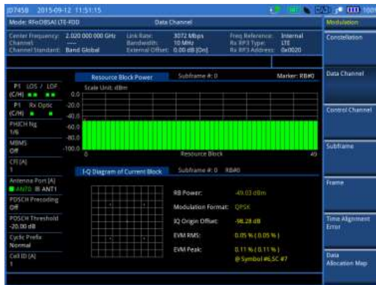
Figure 374 Data channel measurement with RFoBSAI LTE-FDD signal analyzer
