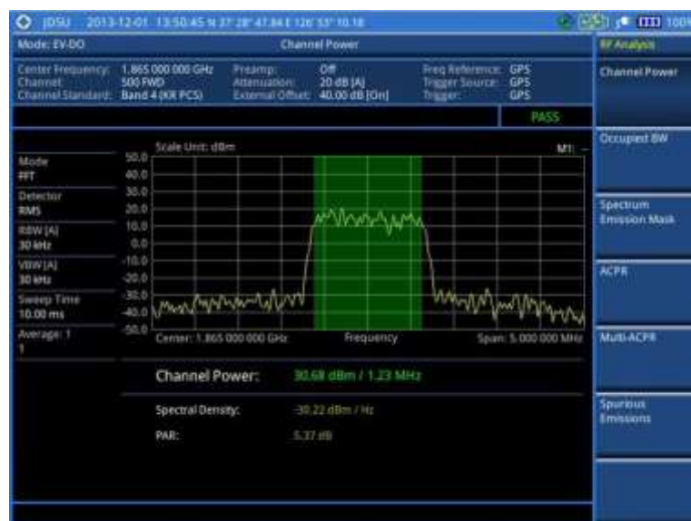
Figure 204 Channel power measurement with EV-DO signal analyzer
