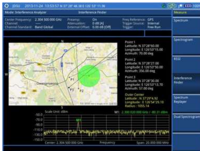
Figure 37 Interference finder measurement in map view
