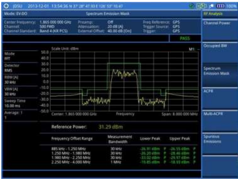
Figure 202 SEM measurement with EV-DO signal analyzer
