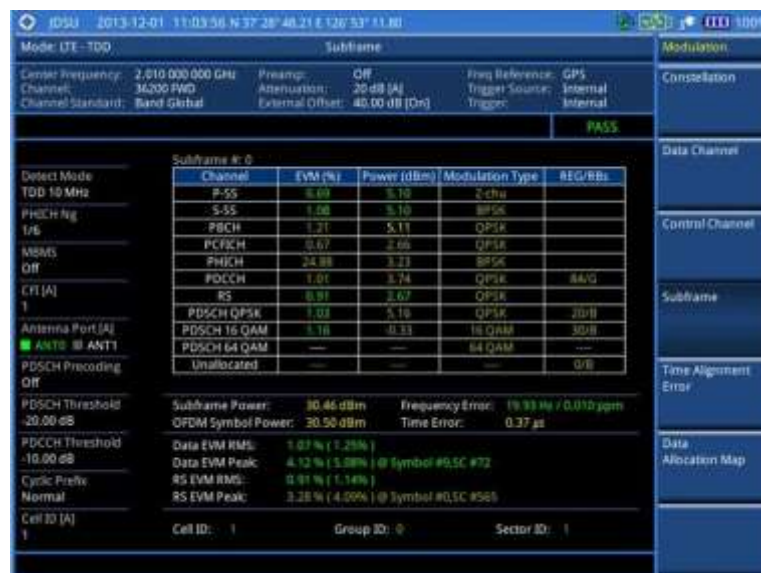
Figure 147 Subframe measurement with LTE-TDD signal analyzer
