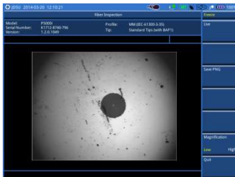
Figure 391 Captured fiber image
