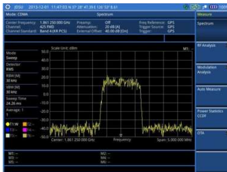
Figure 176 Spectrum measurement screen with CDMA signal analyzer
