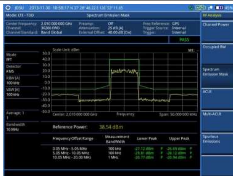
Figure 135 SEM measurement with LTE-TDD signal analyzer
