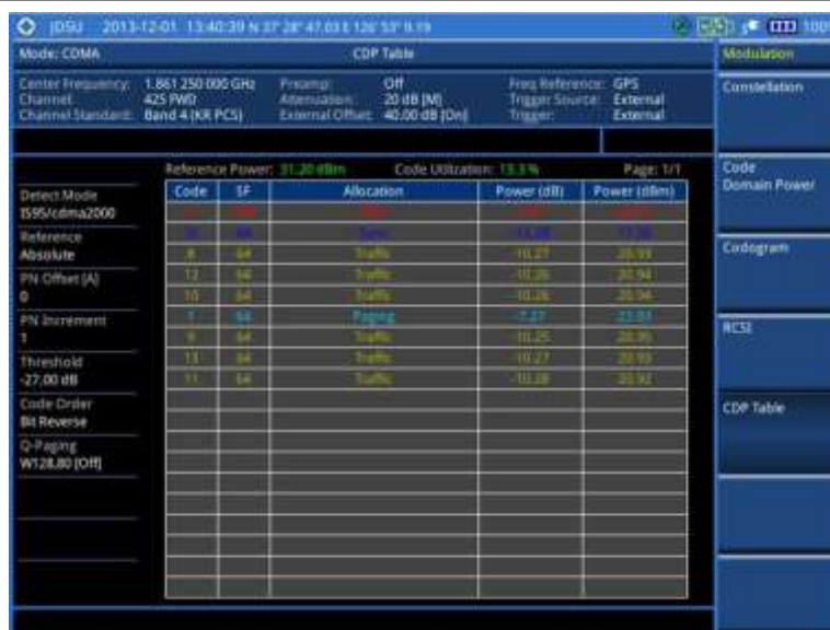
Figure 187 CDP Table measurement with CDMA signal analyzer
