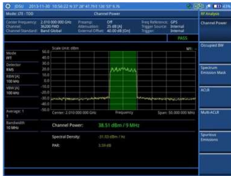
Figure 133 Channel power measurement with LTE-TDD signal analyzer
