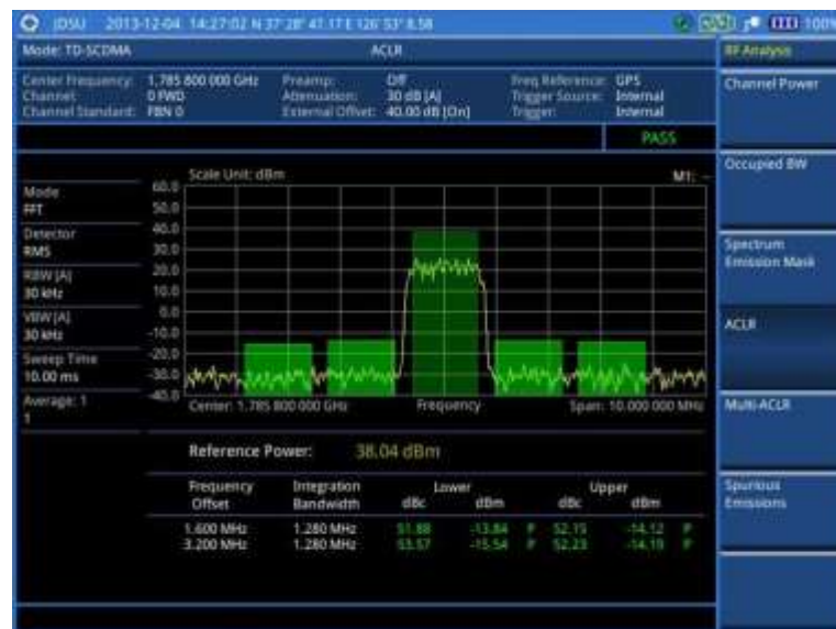
Figure 228 ACLR measurement with TD-SCDMA signal analyzer
