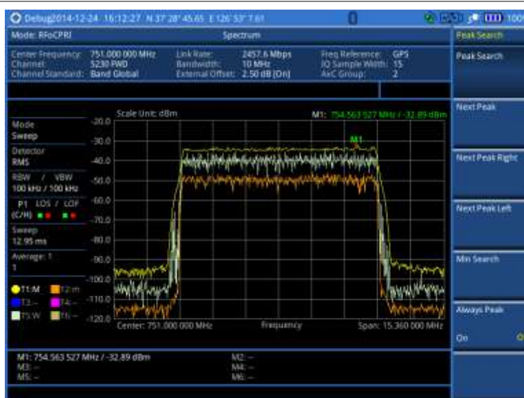
Figure 295 RFoCPRI spectrum analysis on LTE Uplink 10 MHz, antenna 2
