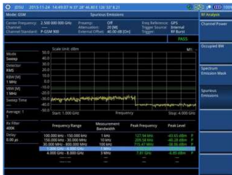
Figure 46 Spurious emissions measurement with GSM signal analyzer
