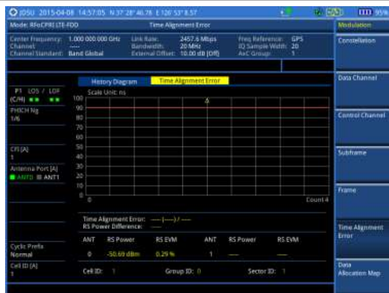
Figure 317 Time alignment error measurement with RFoCPRI LTE-FDD signal analyzer
