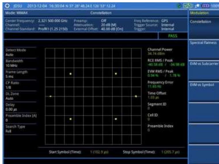
Figure 255 Constellation measurement with Mobile WiMAX signal analyzer
