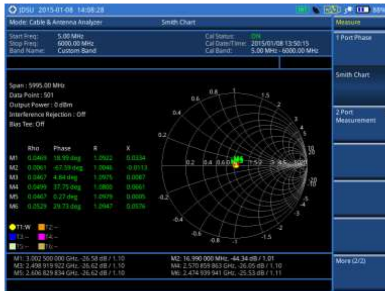
Figure 282 Smith chart measurement
