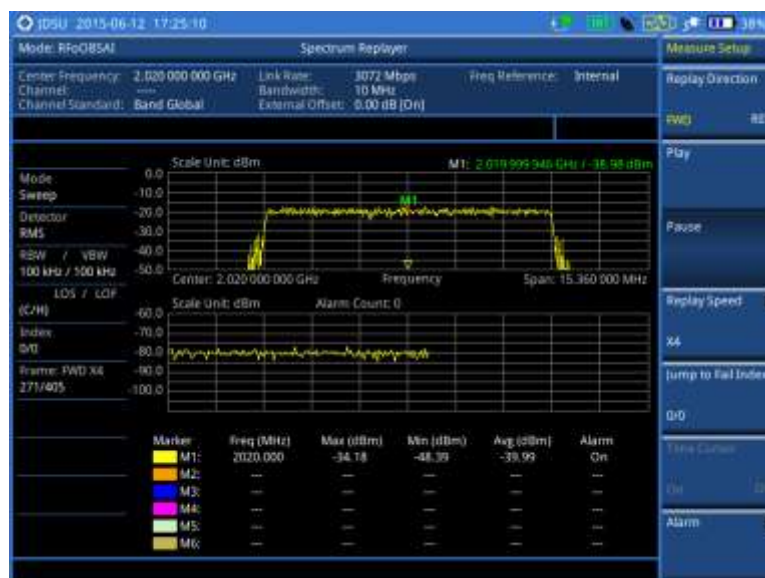
Figure 359 RFoBSAI spectrum replay
