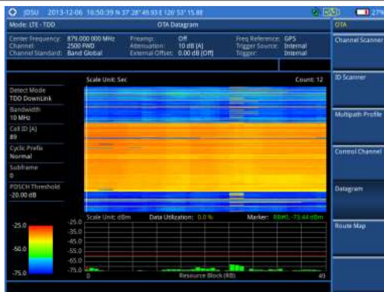
Figure 161 Datagram measurement with LTE-TDD signal analyzer
