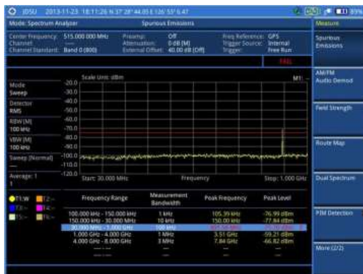
Figure 18 Spurious emissions measurement with spectrum analyzer
