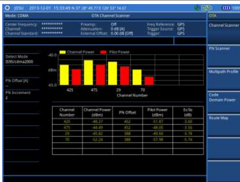
Figure 189 Channel scanner measurement with CDMA OTA signal analyzer
