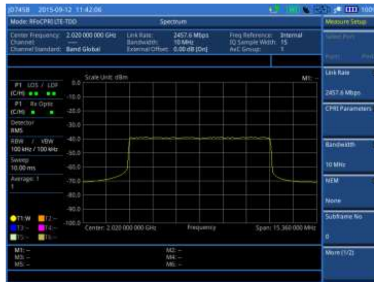
Figure 321 Spectrum measurement with RFoCPRI LTE-TDD signal analyzer
