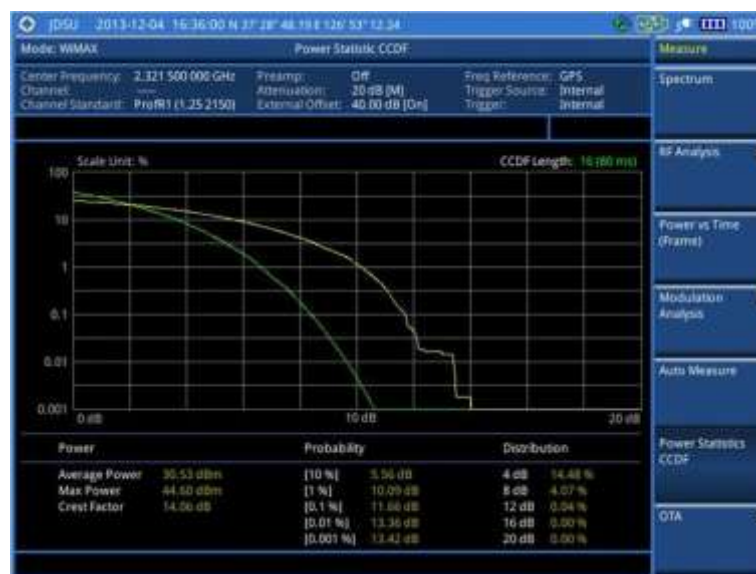
Figure 259 CCDF measurement with Mobile WiMAX signal analyzer
