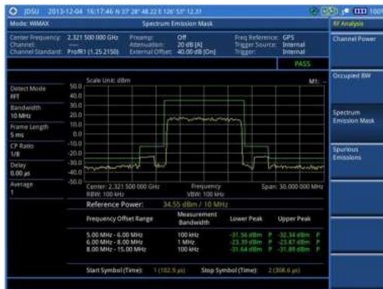
Figure 252 SEM measurement with Mobile WiMAX signal analyzer
