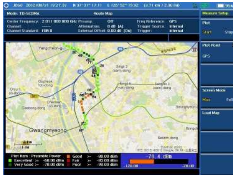
Figure 243 Route map measurement with TD-SCDMA OTA signal analyzer
