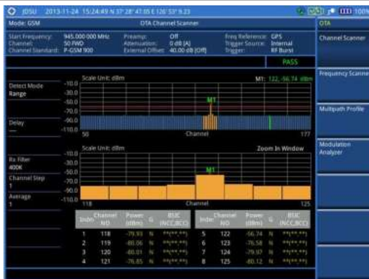
Figure 52 Channel scanner measurement with GSM OTA signal analyzer
