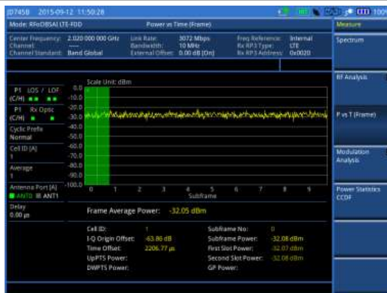
Figure 366 Power vs. time (frame) measurement with RFoOBSAI LTE-FDD signal analyzer
