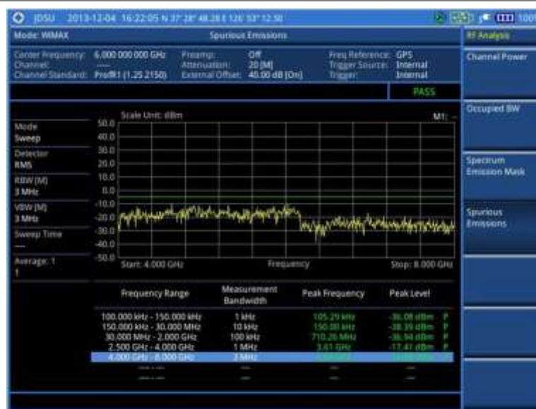
Figure 253 Spurious emissions measurement with Mobile WiMAX signal analyzer
