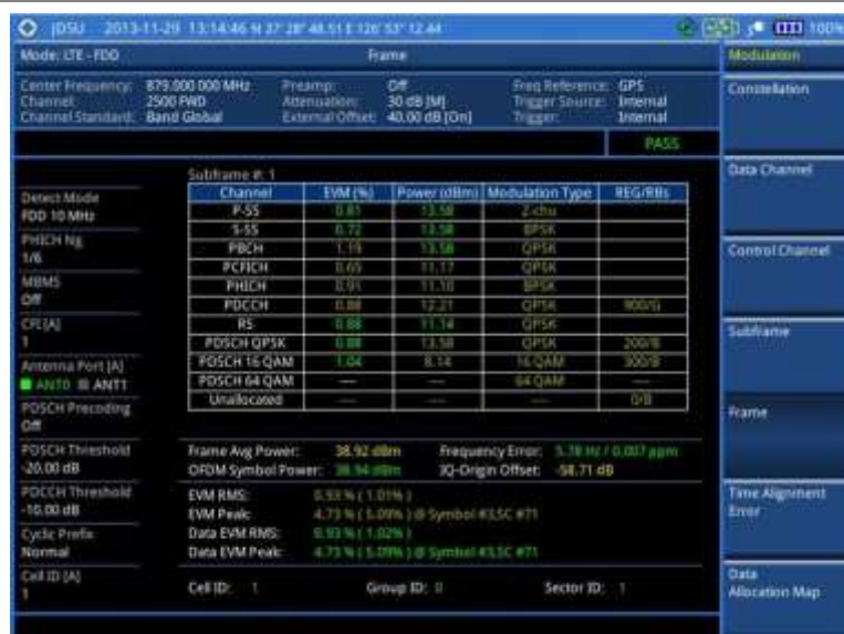
Figure 104 Frame measurement with LTE-FDD signal analyzer
