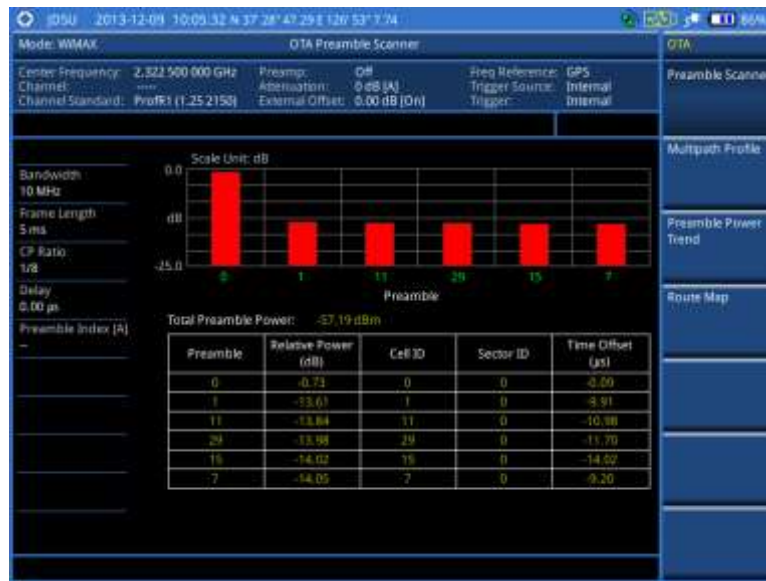
Figure 260 Preamble scanner measurement with Mobile WiMAX OTA signal analyzer
