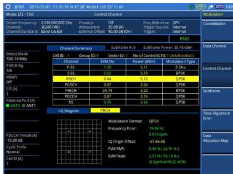
Figure 145 Control channel measurement with LTE-TDD signal analyzer
