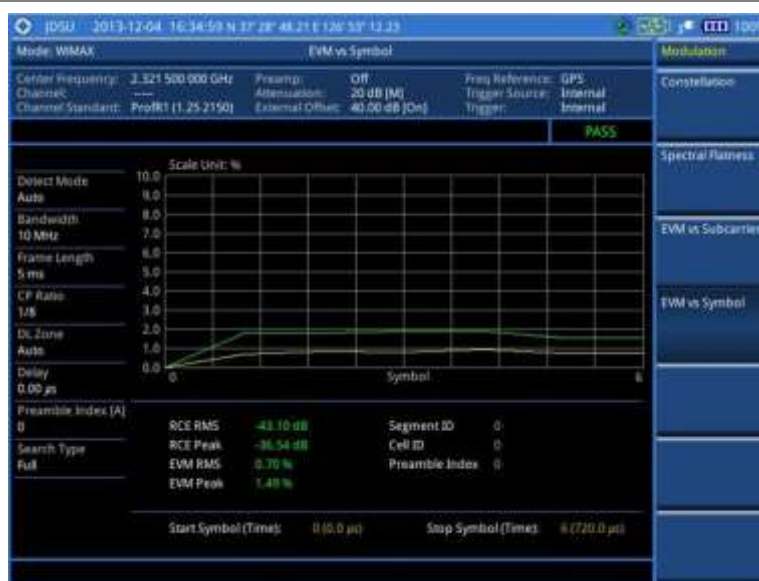
Figure 258 EVM vs. symbol measurement with Mobile WiMAX signal analyzer
