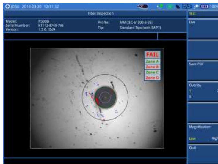
Figure 392 Analyzed fiber image and fiber inspection result
