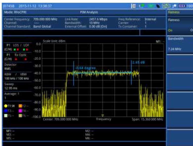
Figure 349 Example of PIM analysis in BBU emulation
