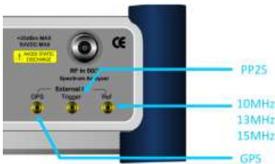
Figure 131 Connection ports for external reference clock
