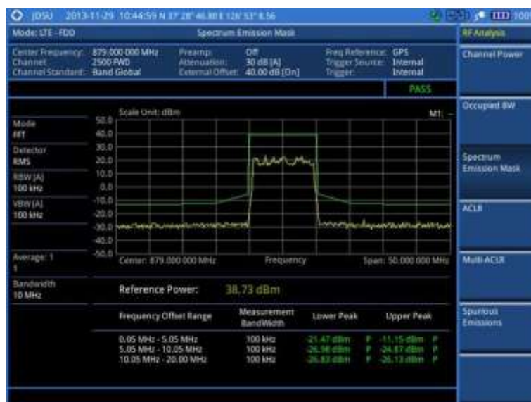
Figure 90 SEM measurement with LTE-FDD signal analyzer
