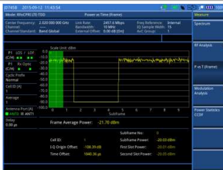
Figure 324 Power vs. time (frame) measurement with RFoCPRI LTE-TDD signal analyzer
