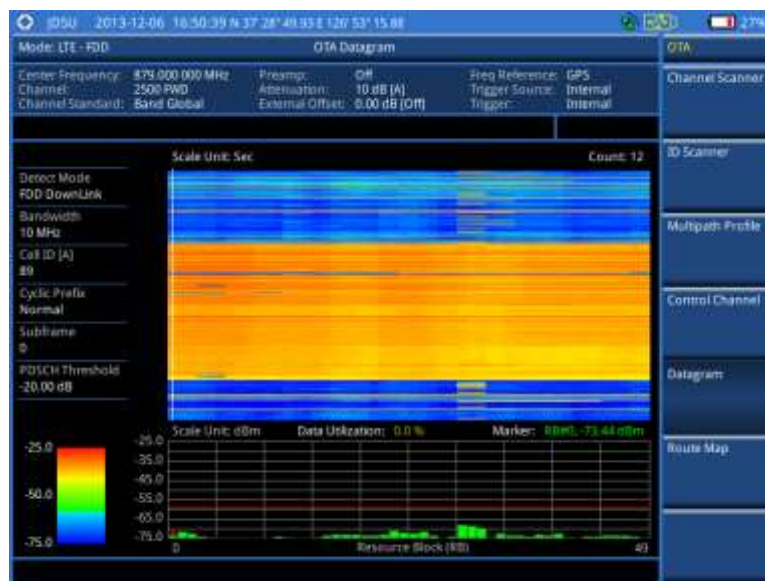
Figure 117 Datagram measurement with LTE-FDD signal analyzer
