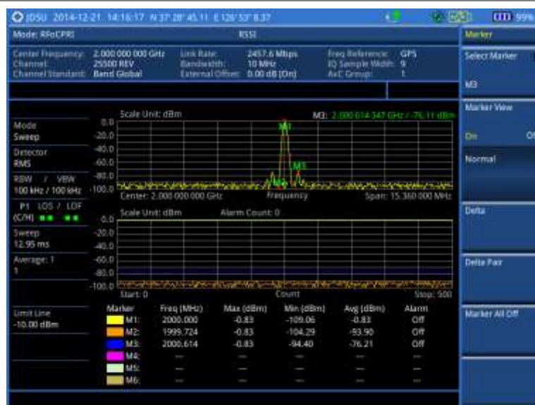
Figure 301 RFoCPRI interference measurement in RSSI
