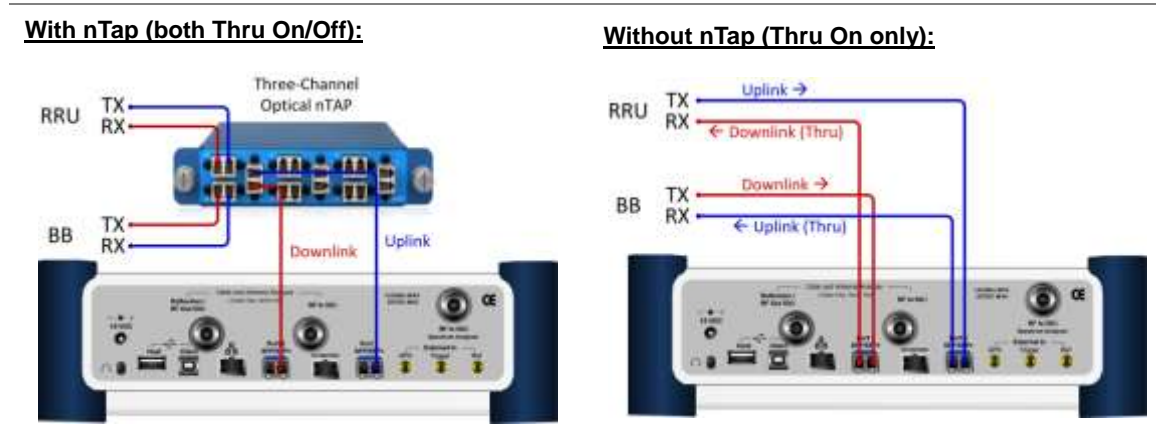
Figure 351 Connection diagram for Layer-2 monitoring mode
