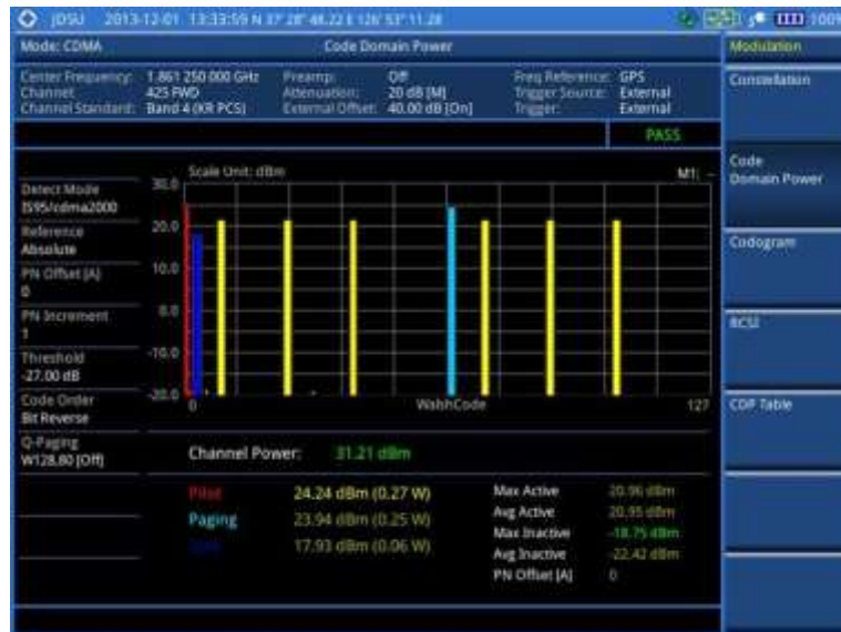
Figure 184 Code domain power measurement with CDMA signal analyzer
