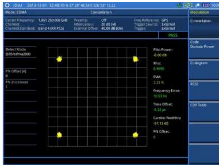
Figure 183 Constellation measurement with CDMA signal analyzer
