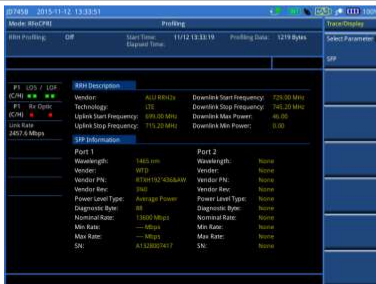
Figure 336 Example of RRH profiling results with SFP information
