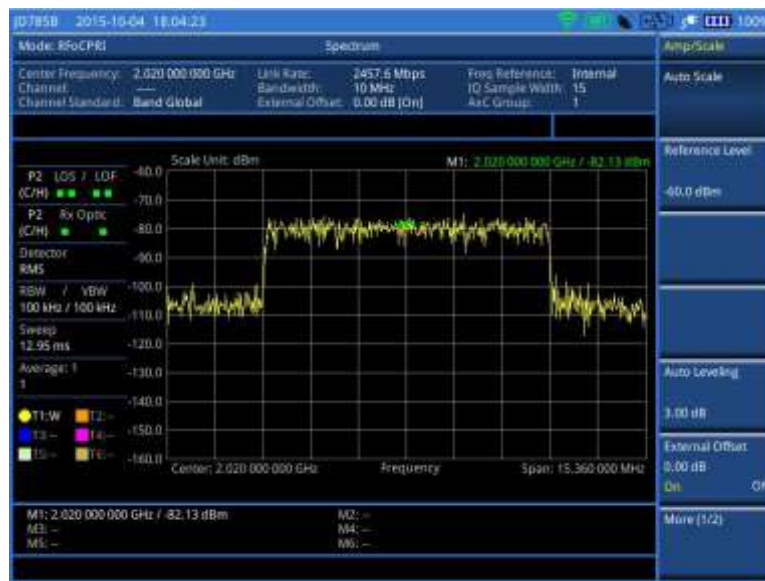
Figure 291 Before enabling Auto Leveling
