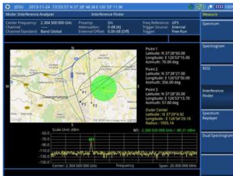
Figure 33 Interference finder measurement in map view
