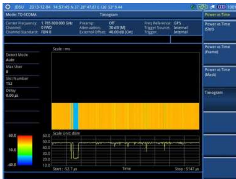
Figure 234 Timogram with TD-SCDMA signal analyzer
