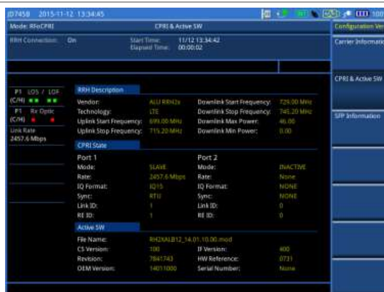
Figure 339 Example of verification of CPRI state and active software
