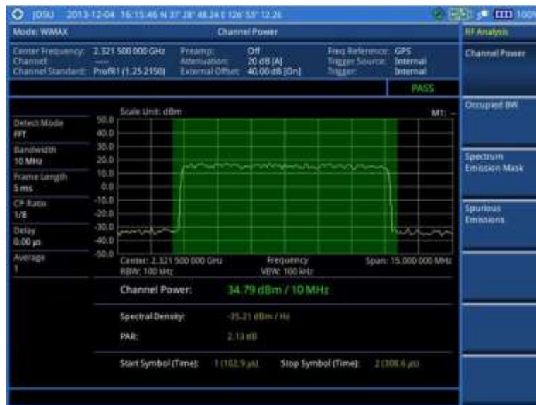
Figure 250 Channel power measurement with Mobile WiMAX signal analyzer
