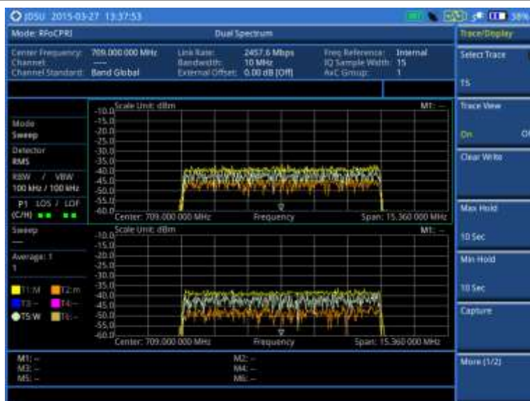
Figure 296 RFoCPRI dual spectrum analysis
