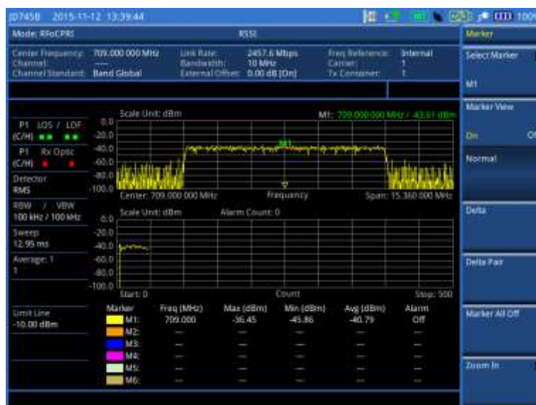
Figure 347 Example of RSSI in BBU emulation
