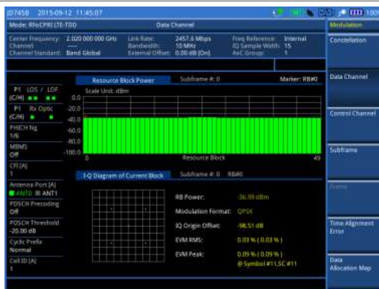
Figure 326 Data channel measurement with RFoCPRI LTE-FDD signal analyzer
