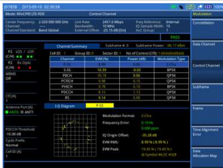
Figure 314 Control channel measurement with RFoCPRI LTE-FDD signal analyzer
