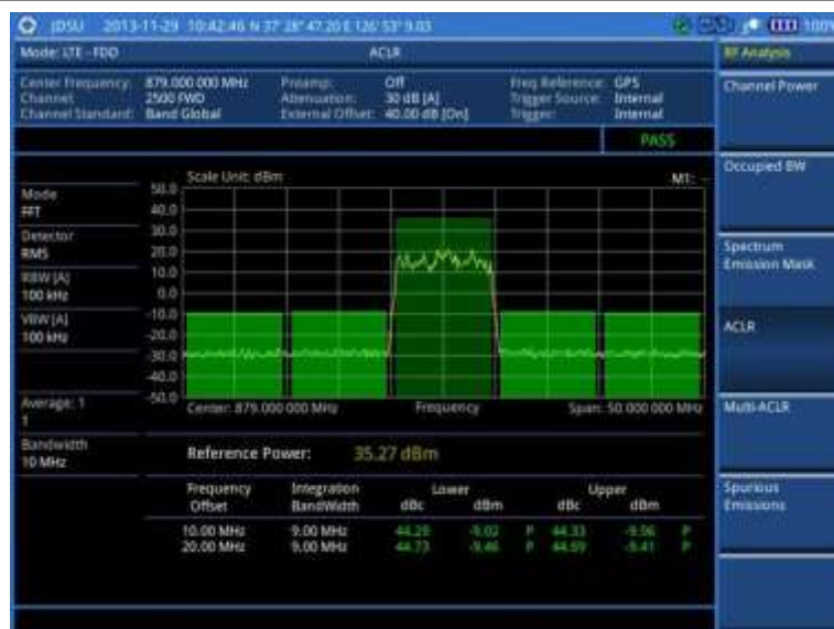
Figure 91 ACLR measurement with LTE-FDD signal analyzer
