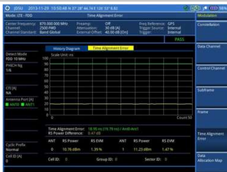
Figure 106 Time alignment error measurement with LTE-FDD signal analyzer
