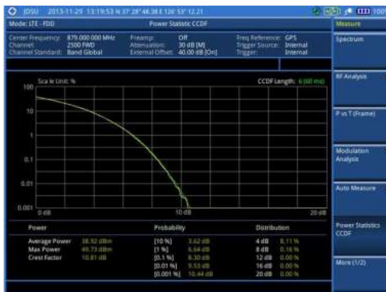
Figure 110 CCDF measurement with LTE-FDD signal analyzer
