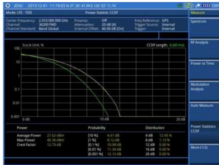
Figure 154 CCDF measurement with LTE-TDD signal analyzer
