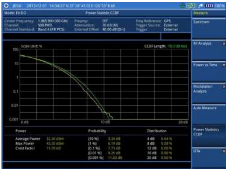
Figure 213 CCDF measurement with EV-DO signal analyzer
