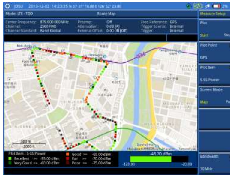
Figure 168 Route map measurement (S-SS Ec/Io) with LTE-TDD OTA signal analyzer
