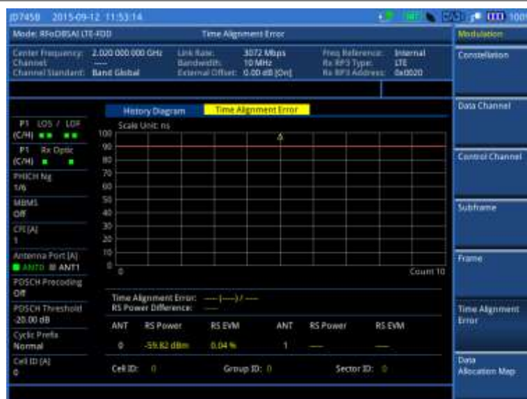
Figure 372 Time alignment error measurement with RFoBSAI LTE-FDD signal analyzer
