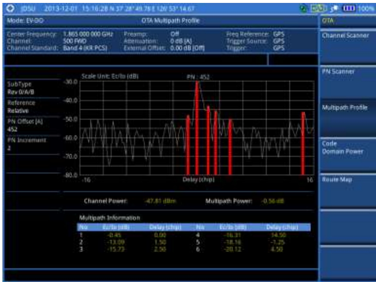
Figure 216 Multipath profile measurement with EV-DO OTA signal analyzer
