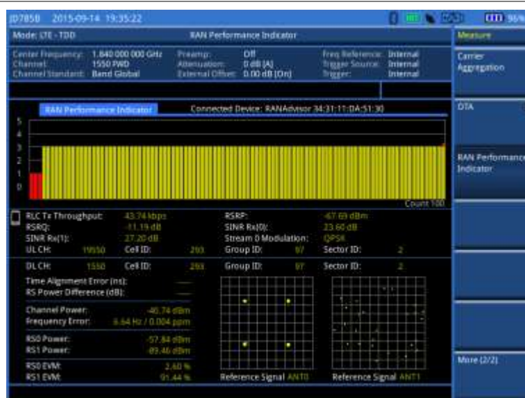
Figure 170 RAN performance indicator with LTE-TDD signal analyzer
