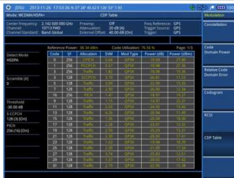
Figure 73 CDP Table measurement with WCDMA/HSPA+ signal analyzer
