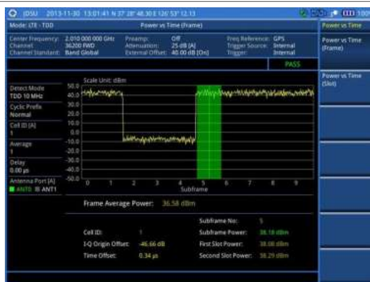
Figure 140 Power vs. time (frame) measurement with LTE – TDD signal analyzer
