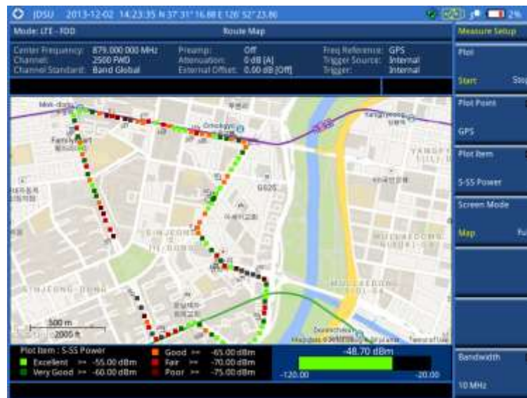
Figure 123 Route map measurement (S-SS Power) with LTE-FDD OTA signal analyzer
