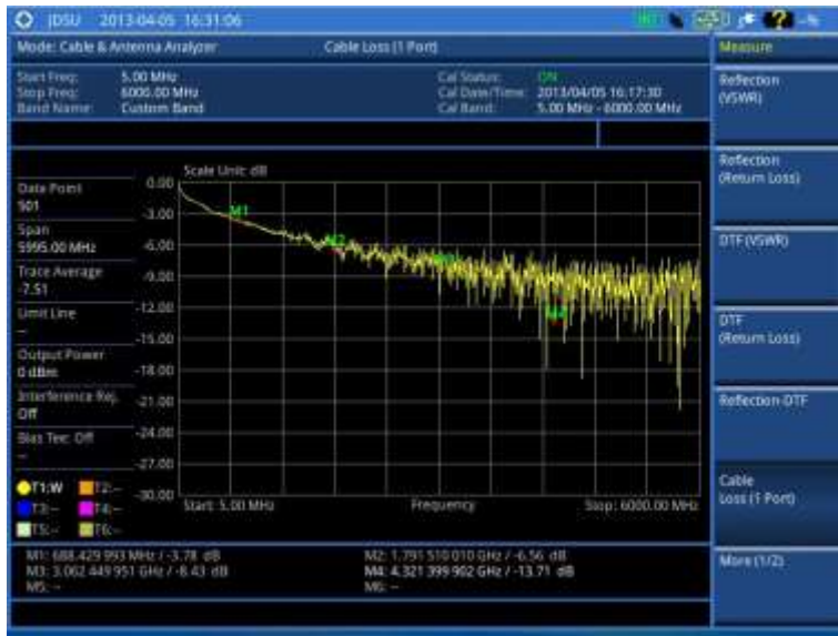
Figure 278 Cable loss (1 port) measurement
