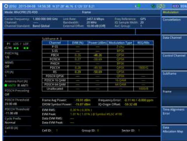
Figure 316 Frame measurement with RFoCPRI LTE-FDD signal analyzer
