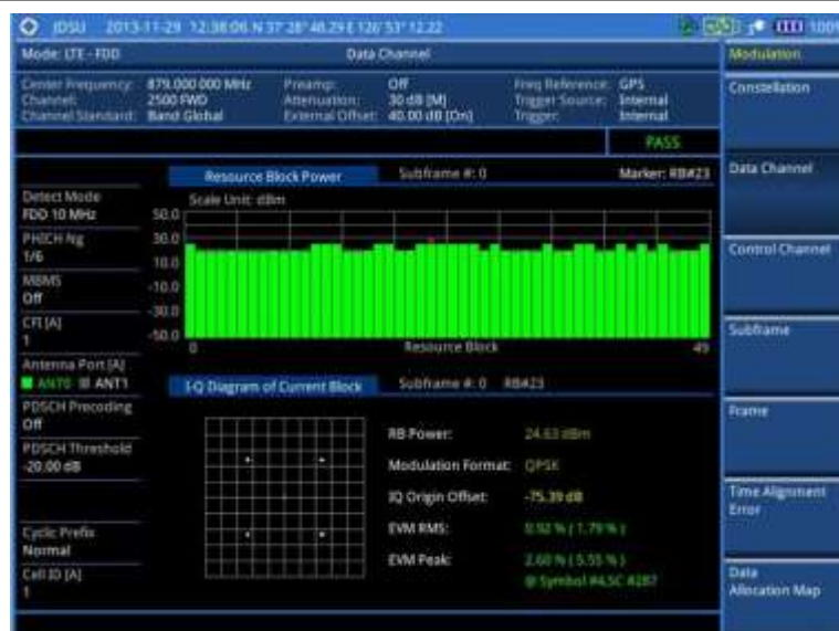
Figure 97 Data channel measurement with LTE-FDD signal analyzer
