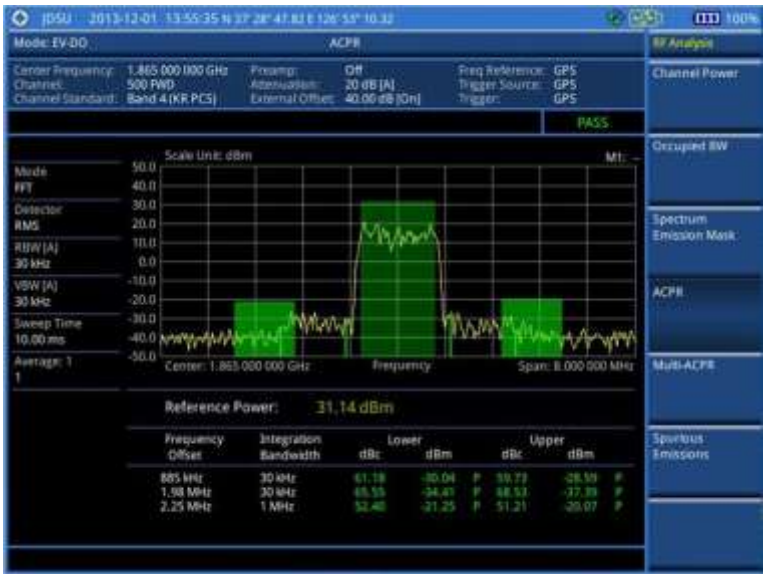
Figure 203 ACPR measurement with EV-DO signal analyzer
