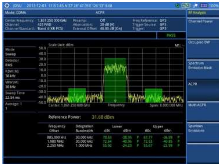
Figure 180 ACPR measurement with CDMA signal analyzer
