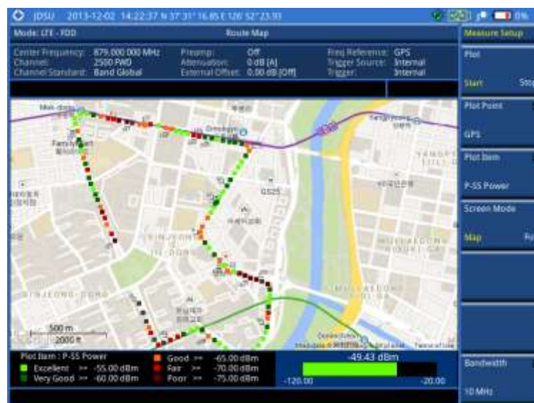
Figure 122 Route map measurement (P-SS Power) with LTE-FDD OTA signal analyzer
