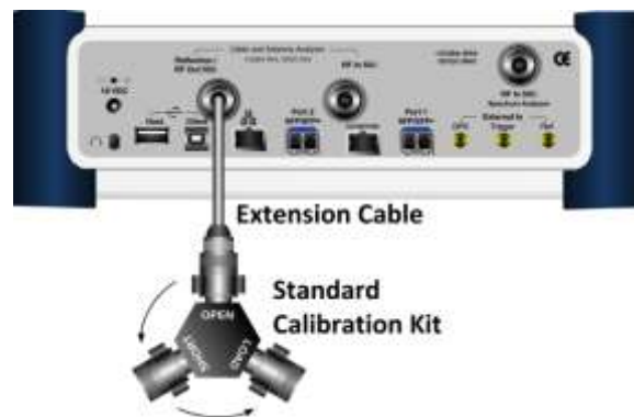
Figure 265 1-port calibration connection with mechanical Y-Cal kit
