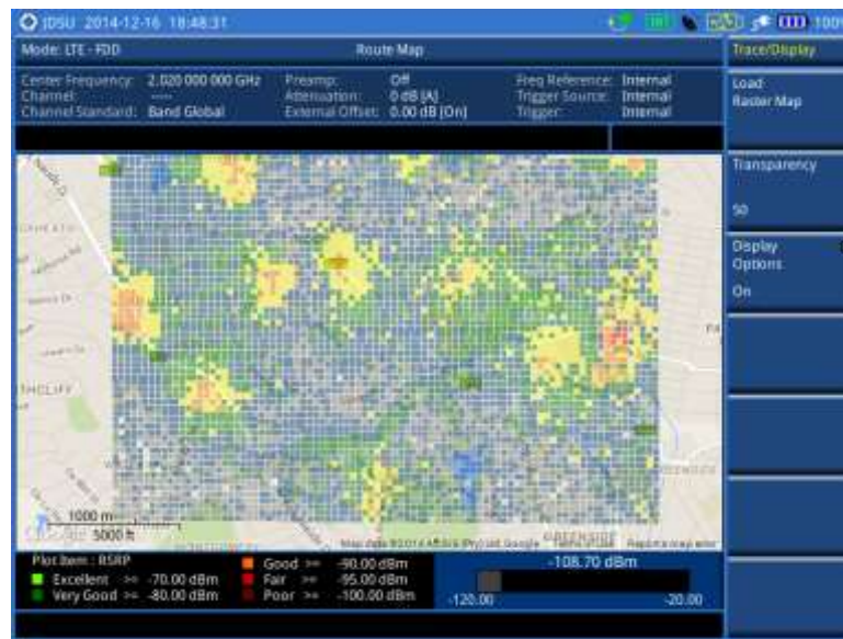
Figure 125 Raster image overlaid on the base map with LTE-FDD OTA signal analyzer
