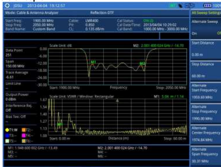
Figure 277 Reflection-DTF dual measurement
