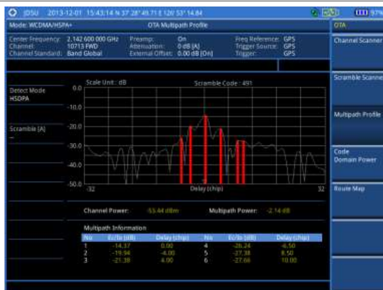
Figure 77 Multipath profile measurement with WCDMA/HSPA+ OTA signal analyzer
