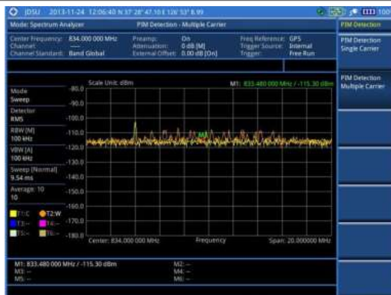
Figure 25 PIM detection for multiple carriers
