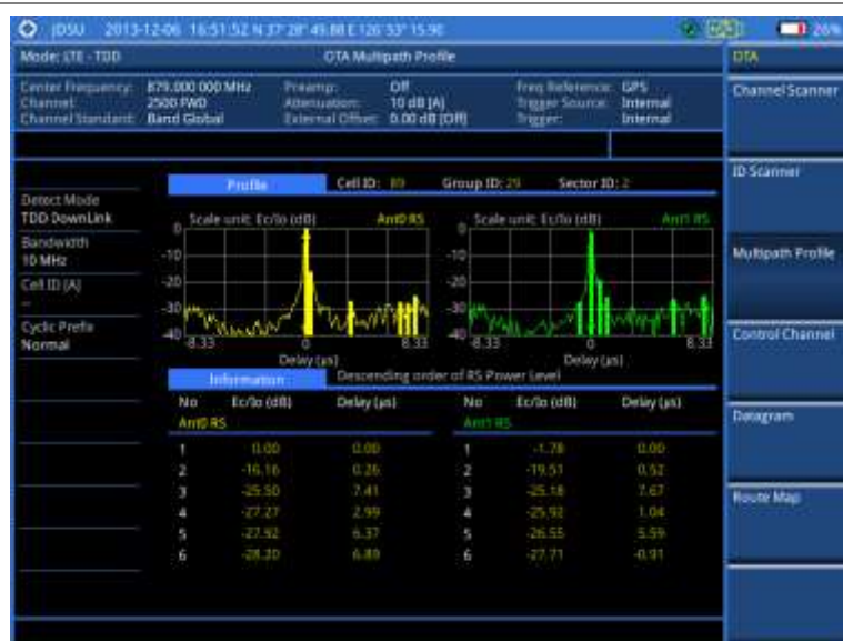
Figure 159 Multipath profile measurement with LTE-TDD OTA signal analyzer
