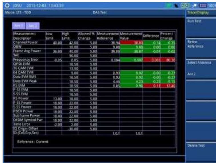
Figure 153 DAS measurement with LTE-TDD signal analyzer
