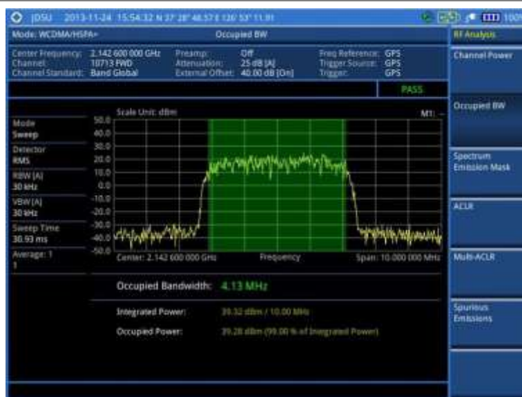
Figure 63 Occupied bandwidth measurement with WCDMA/HSPA+ signal analyzer
