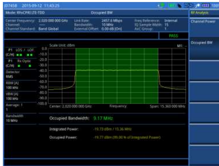
Figure 323 Occupied bandwidth measurement with RFoCPRI LTE-TDD signal analyzer
