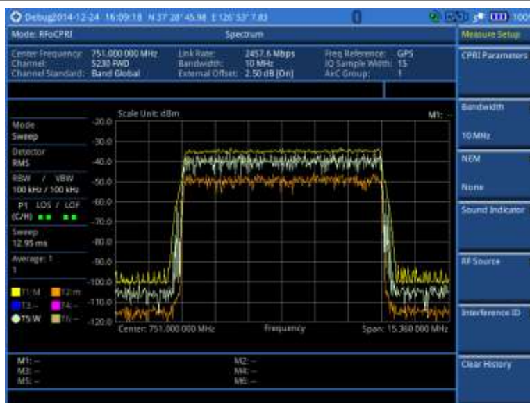
Figure 295 RFoCPRI spectrum analysis on LTE Uplink 10 MHz, antenna 2
