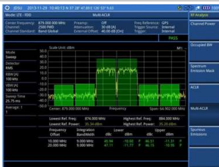
Figure 92 Multi-ACLR measurement with LTE-FDD signal analyzer
