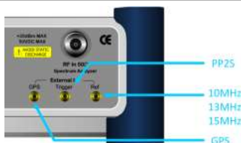
Figure 86 Connection ports for external reference clock
