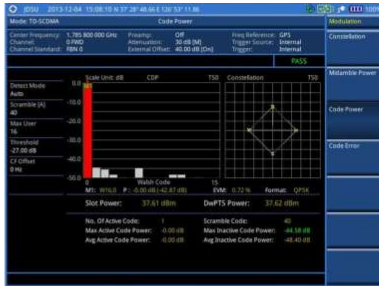
Figure 237 Code power measurement with TD-SCDMA signal analyzer
