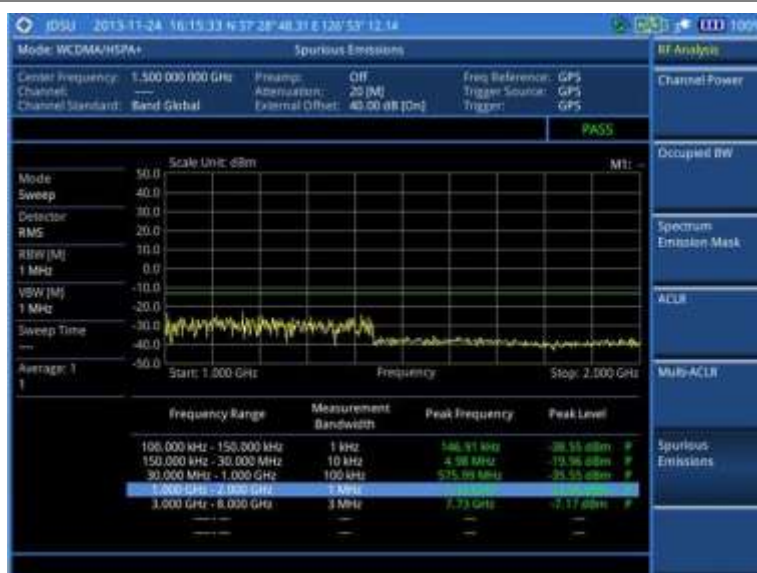
Figure 67 Spurious emissions measurement with WCDMA/HSPA+ signal analyzer
