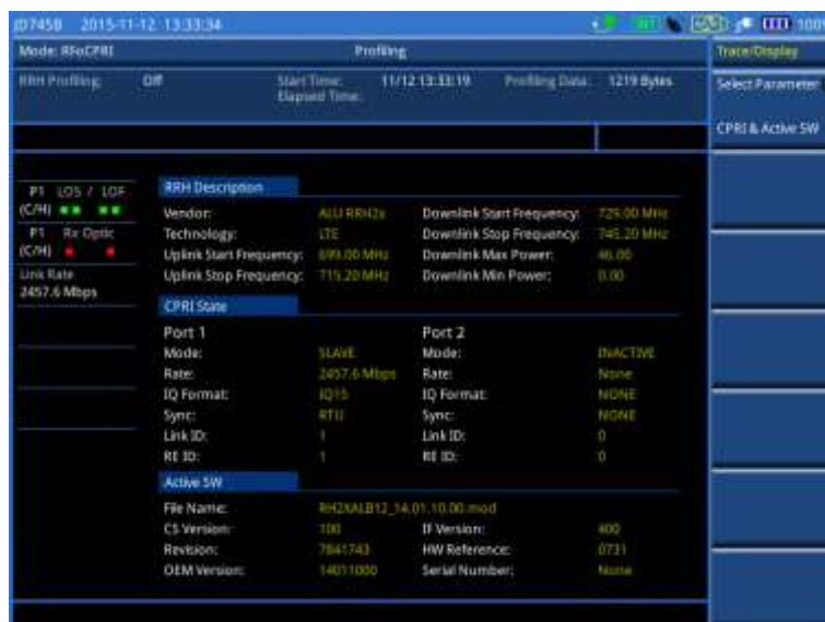
Figure 336 Example of RRH profiling results with SFP information
