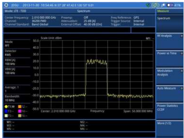
Figure 132 Spectrum measurement screen with LTE-TDD signal analyzer
