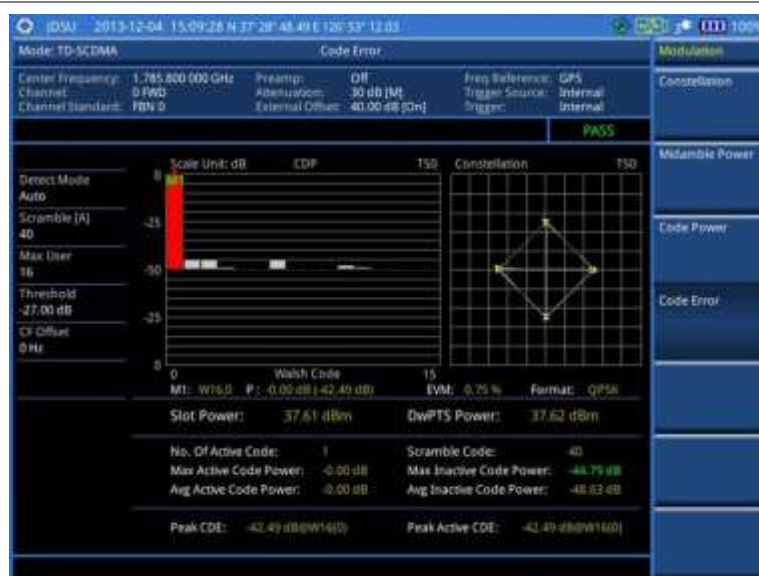
Figure 238 Code error measurement with TD-SCDMA signal analyzer
