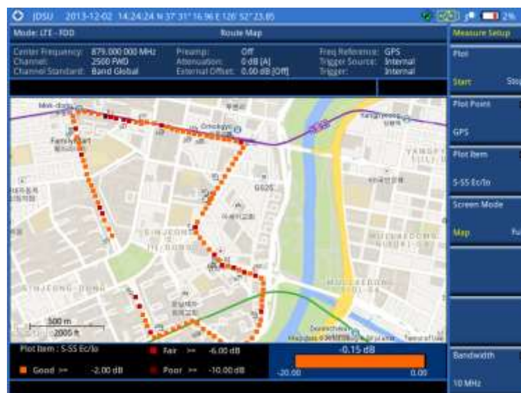
Figure 124 Route map measurement (S-SS Ec/Io) with LTE-FDD OTA signal analyzer
