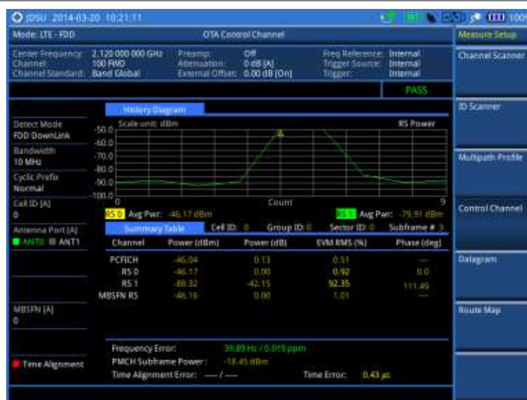
Figure 116 Control channel measurement with LTE-FDD OTA signal analyzer
