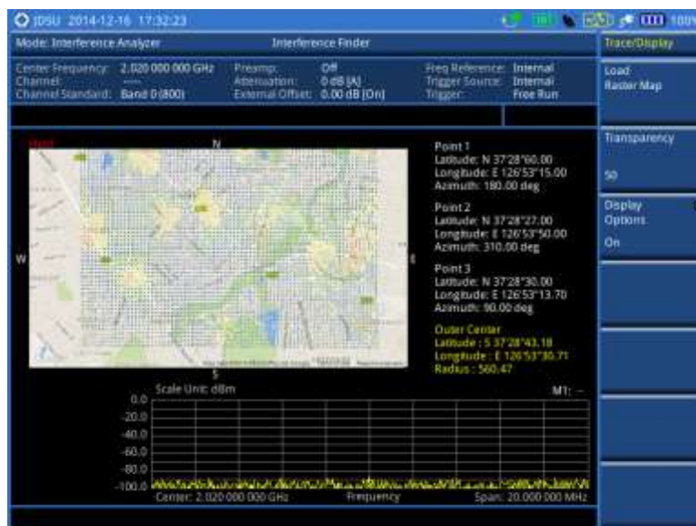
Figure 34 Raster image overlaid on the map in interference finder
