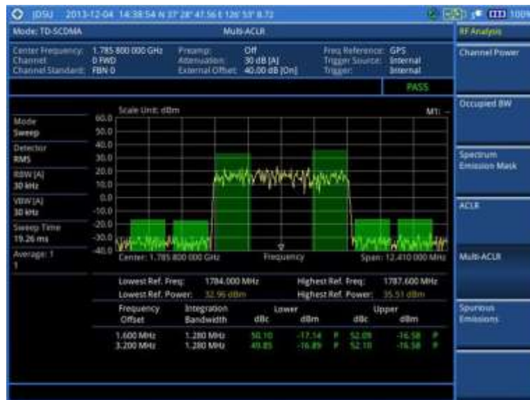
Figure 229 Multi-ACLR measurement with TD-SCDMA signal analyzer
