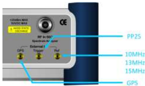
Figure 248 Connection ports for external reference clock
