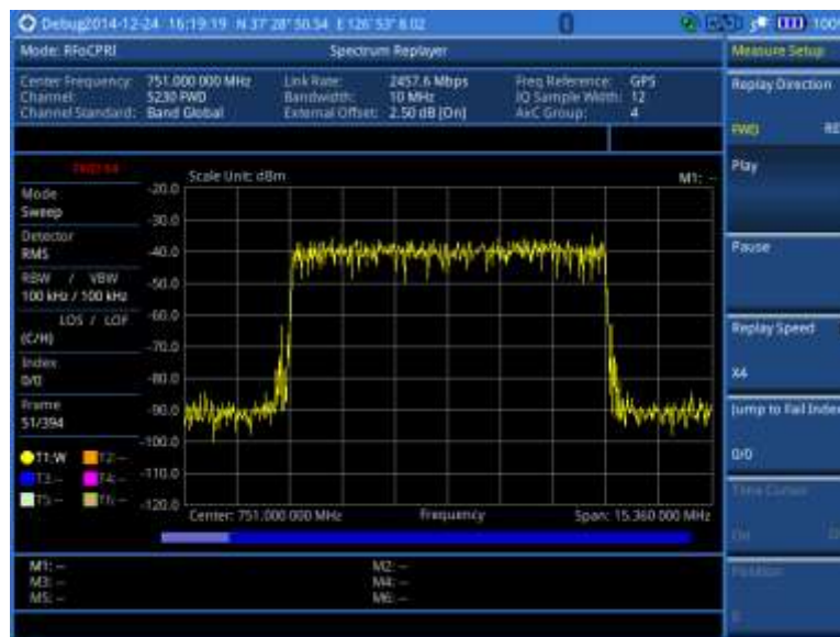
Figure 303 RFoCPRI spectrum replay
