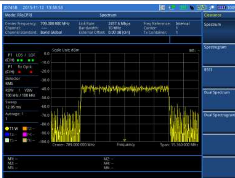
Figure 343 Example of spectrum measurement in BBU emulation
