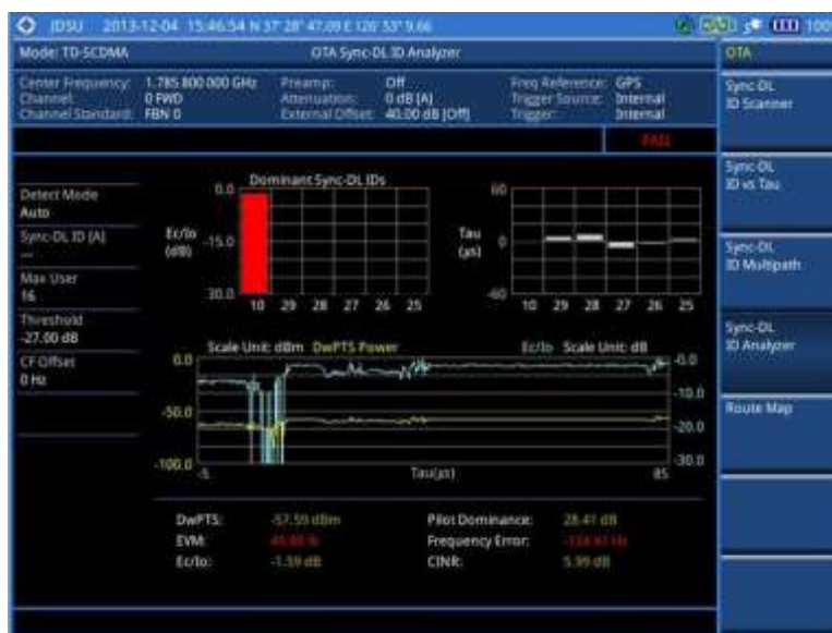
Figure 242 Sync-DL ID analyzer measurement with TD-SCDMA OTA signal analyzer
