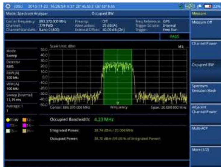
Figure 14 Occupied bandwidth measurement with spectrum analyzer
