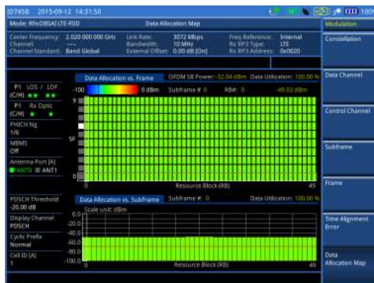
Figure 373 Data allocation map measurement with RFoBSAI LTE-FDD signal analyzer
