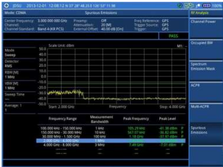
Figure 182 Spurious emissions measurement with CDMA signal analyzer
