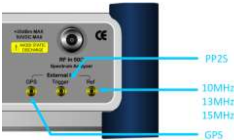
Figure 223 Connection ports for external reference clock
