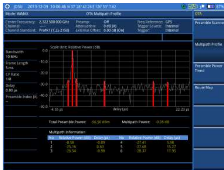
Figure 261 Multipath profile measurement with Mobile WiMAX OTA signal analyzer
