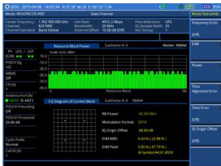
Figure 313 Data channel measurement with RFoCPRI LTE-FDD signal analyzer
