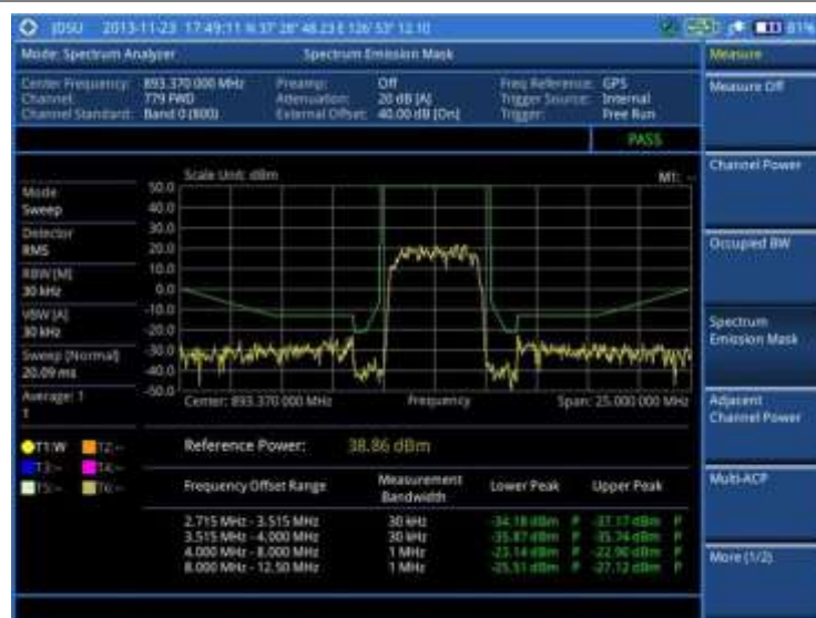
Figure 15 Spectrum emission mask measurement with spectrum analyzer
