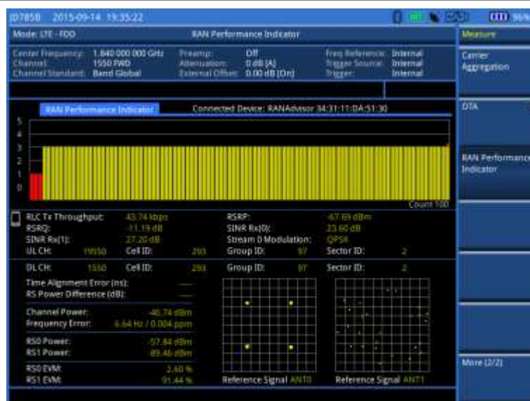
Figure 126 RAN performance indicator with LTE-FDD signal analyzer
