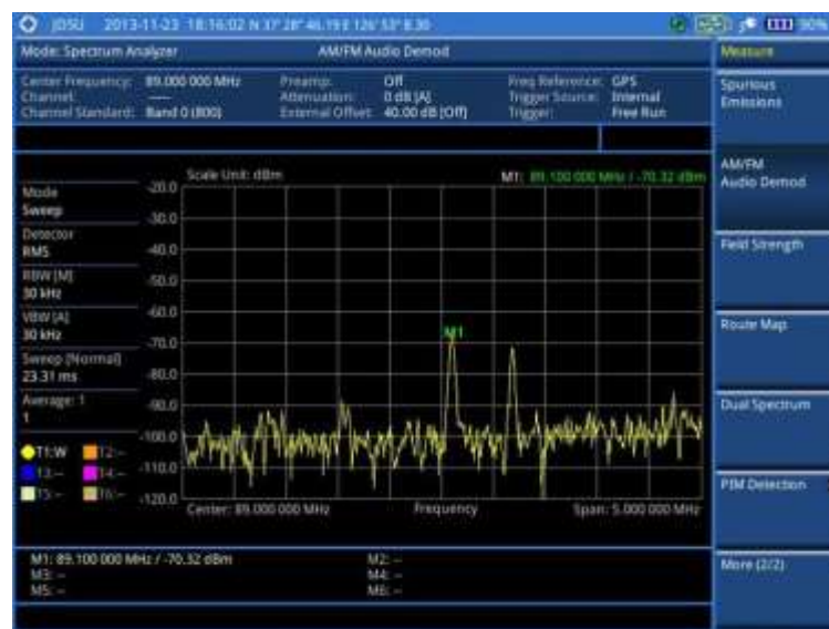
Figure 19 AM/FM audio demodulation with spectrum analyzer
