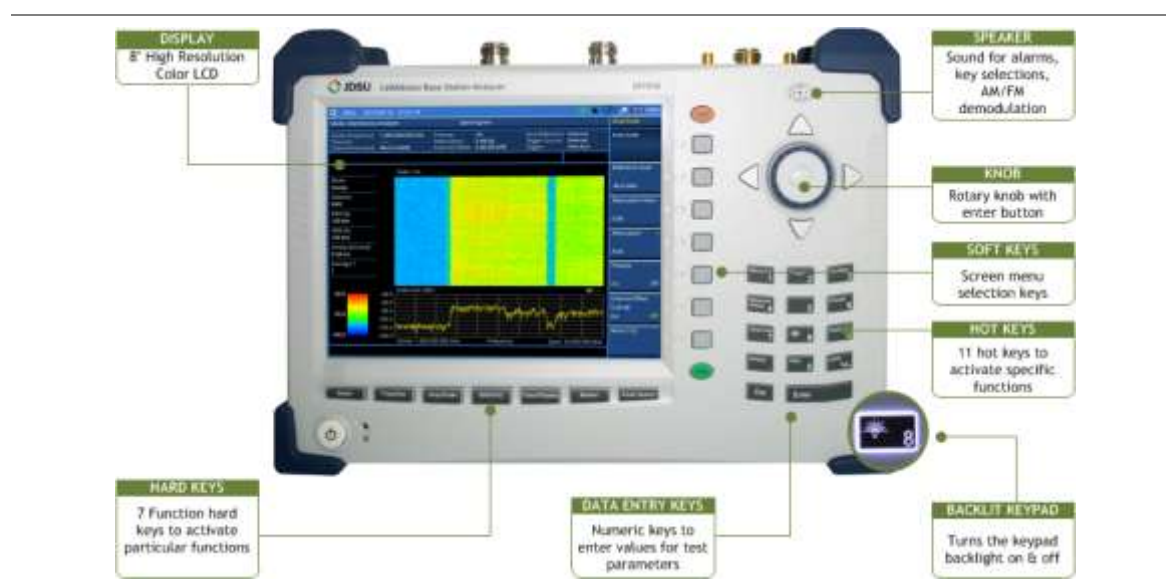
Figure 1 JD785B front panel view
