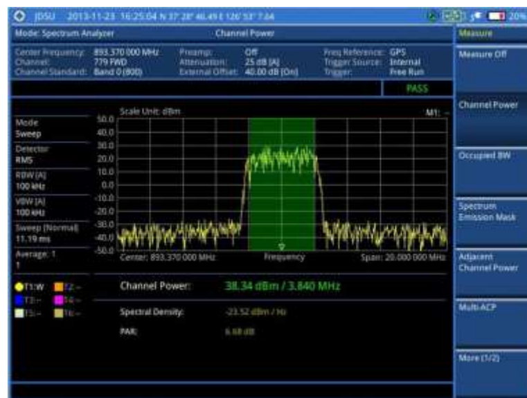
Figure 13 Channel power measurement with spectrum analyzer
