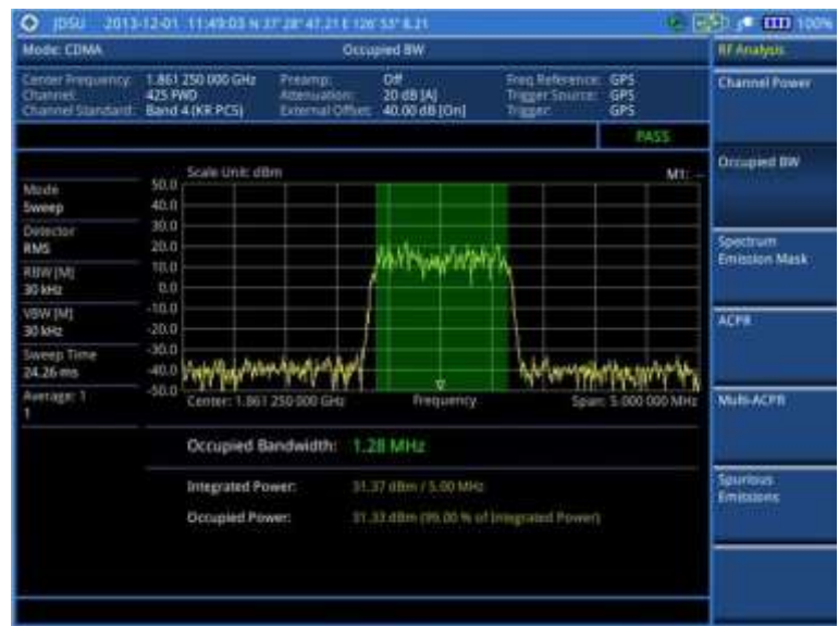
Figure 178 Occupied bandwidth measurement with CDMA signal analyzer
