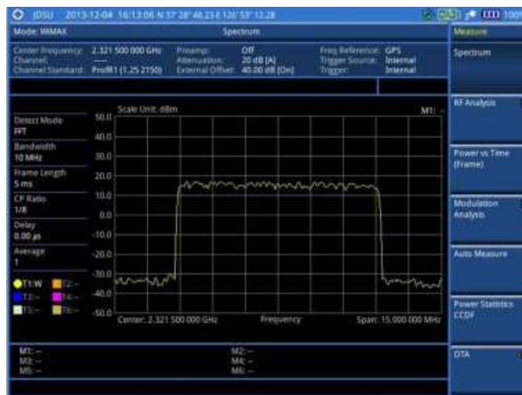
Figure 249 Spectrum measurement screen with Mobile WiMAX signal analyzer
