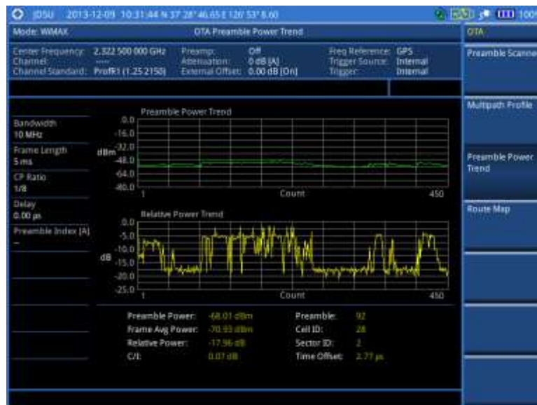
Figure 262 Preamble power trend with Mobile WiMAX OTA signal analyzer
