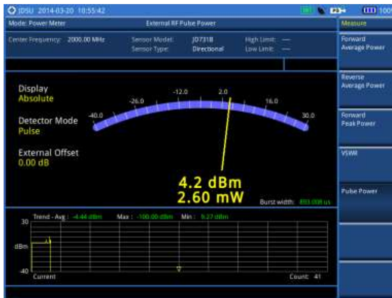
Figure 387 External power measurement of pulse power
