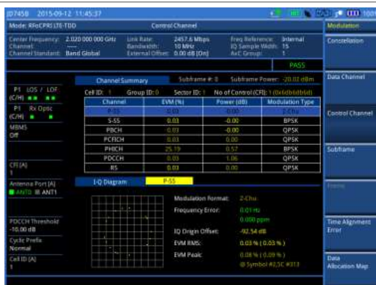
Figure 327 Control channel measurement with RFoCPRI LTE-TDD signal analyzer
