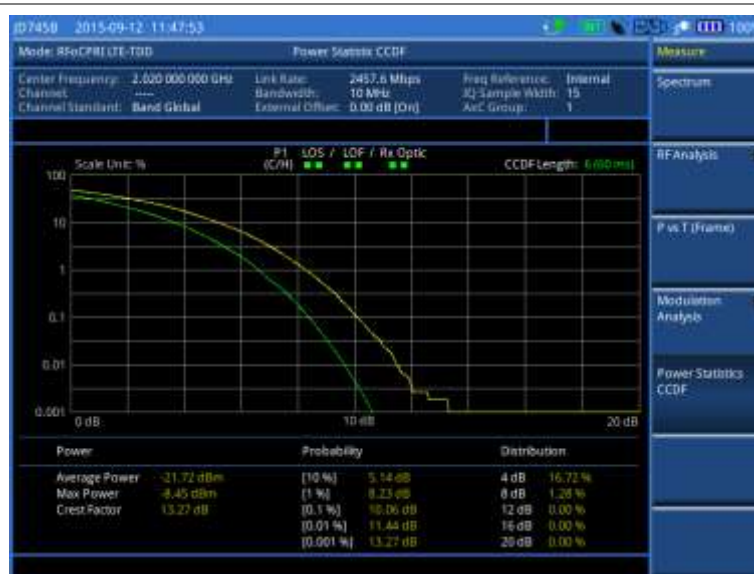
Figure 331 CCDF measurement with RFoCPRI LTE-TDD signal analyzer
