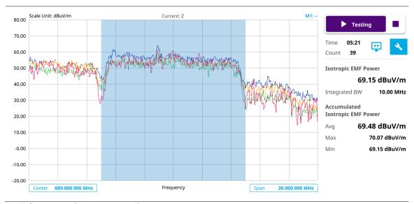
EMF Spectrum (level recorder) measurement
